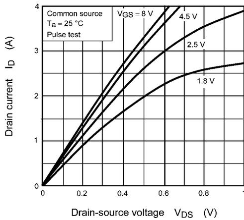
**Fig. 7.1.1**  $I_D - V_{DS}$
