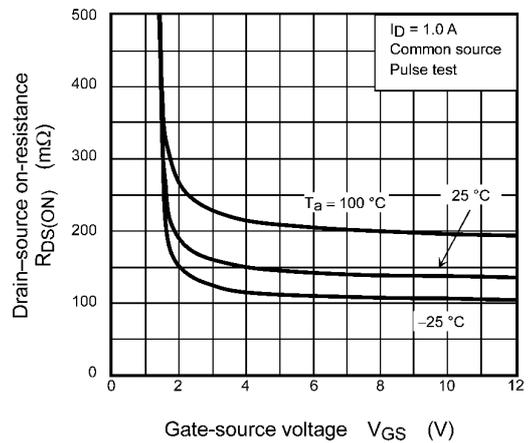
**Fig. 7.1.4**  $R_{DS(ON)} - V_{GS}$
