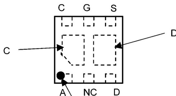
Polarity marking (on the top)
