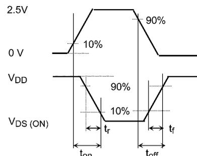
Fig. 5.2.2 Input Waveform/Output Waveform
