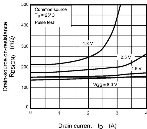
**Fig. 7.1.5**  $R_{DS(ON)} - I_D$
