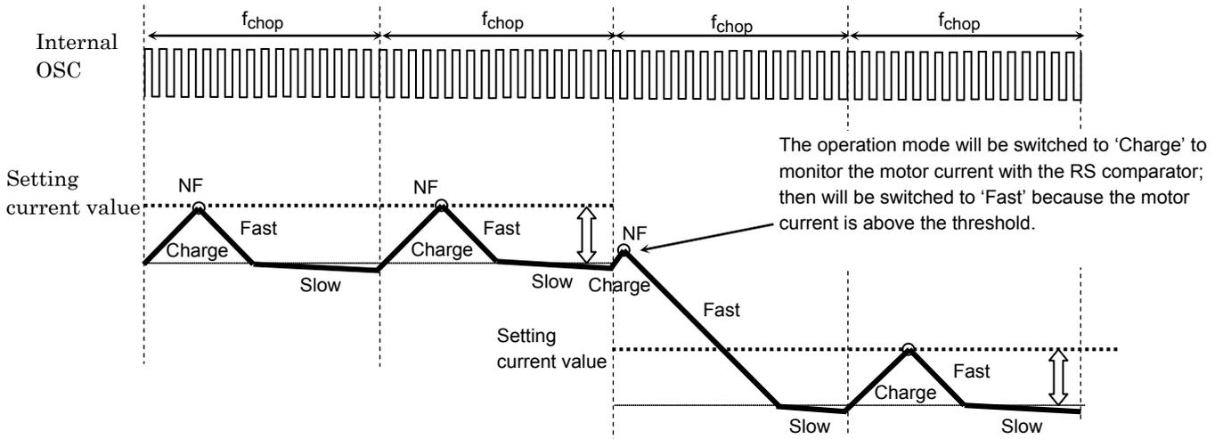
**•When the Fast continues past 1 f\_chop cycle (the motor current not reaching the ADMD threshold during 1 f\_chop cycle)**
