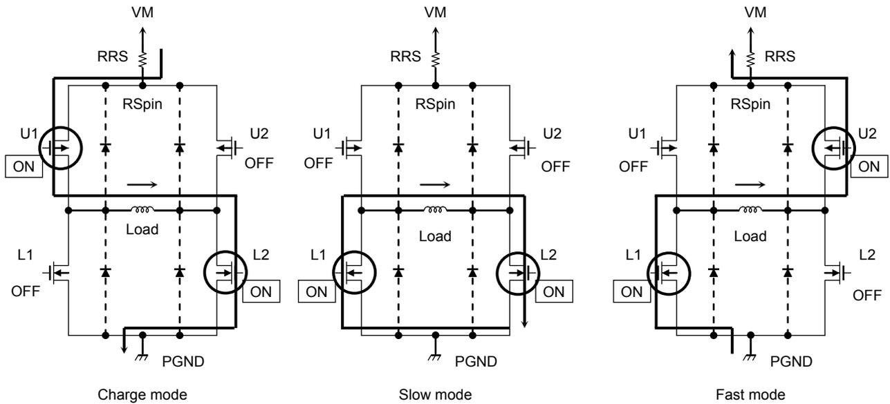
**Output transistor function**
