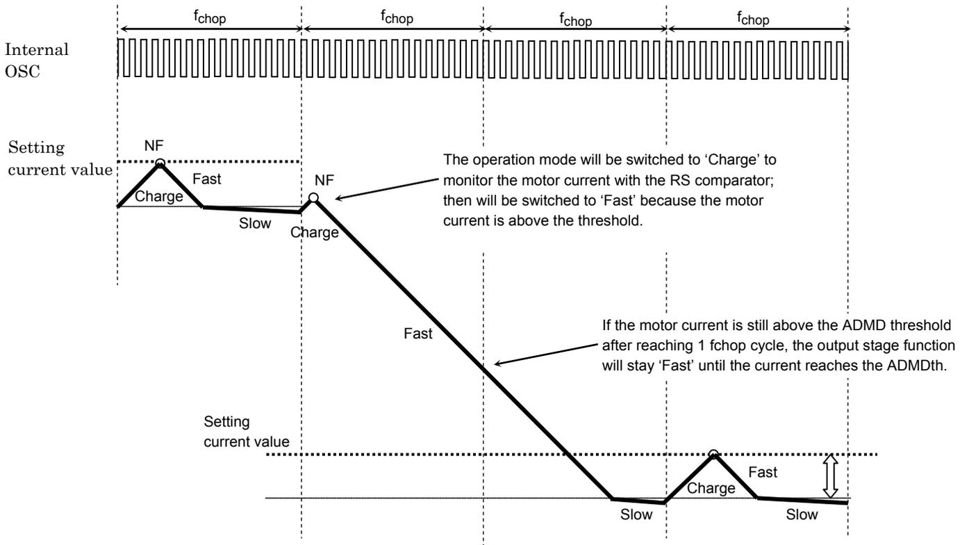
**7. Output transistor function mode**
