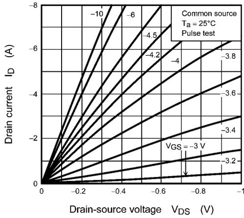
**Fig. 8.2.1  $I_D - V_{DS}$**
