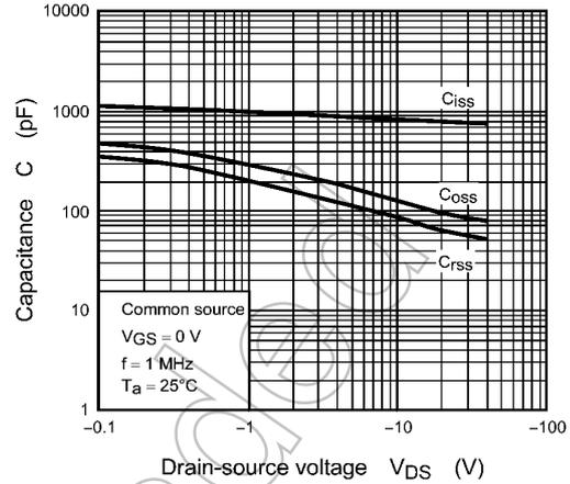
Fig. 8.2.8 Capacitance -  $V_{DS}$
