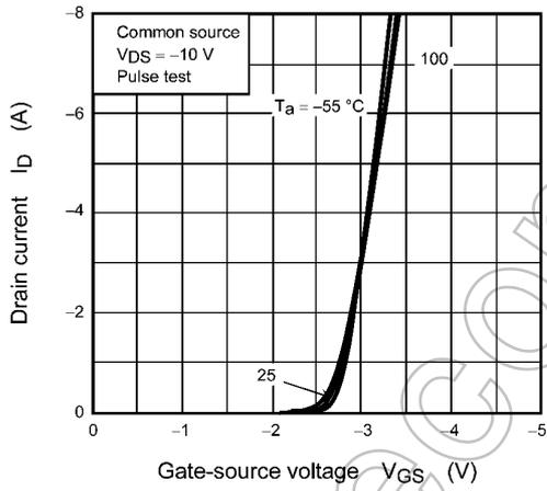
**Fig. 8.2.3  $I_D - V_{GS}$**
