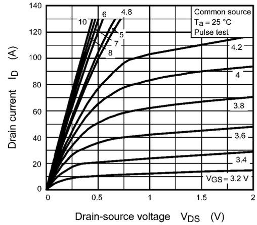
Fig. 8.2  $I_D - V_{DS}$
