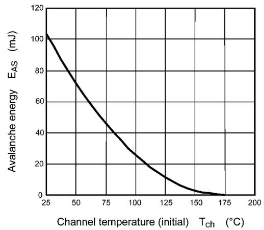
**Fig. 8.14**  $E_{AS} - T_{ch}$
