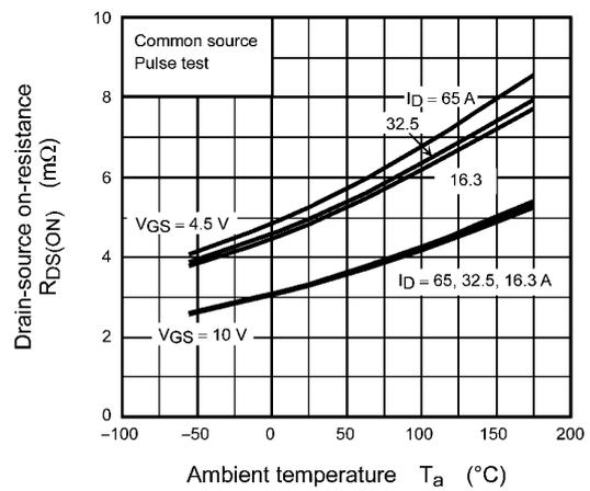
Fig. 8.6  $R_{DS(ON)} - T_a$
