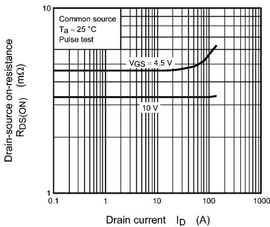
Fig. 8.5  $R_{DS(ON)} - I_D$
