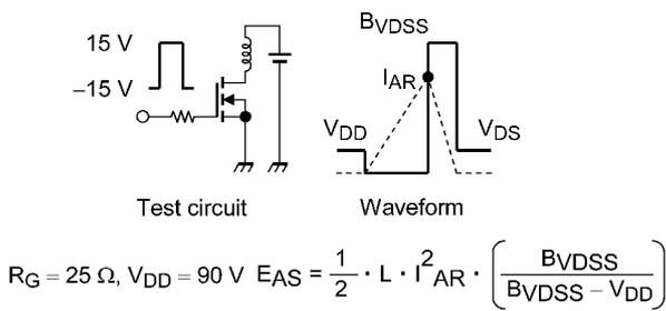
**Fig. 8.16 Test Circuit/Waveform**
