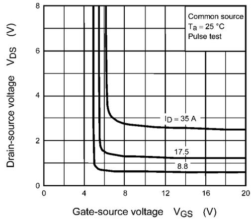
**Fig. 8.4  $V_{DS} - V_{GS}$**
