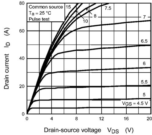
**Fig. 8.2  $I_D - V_{DS}$**
