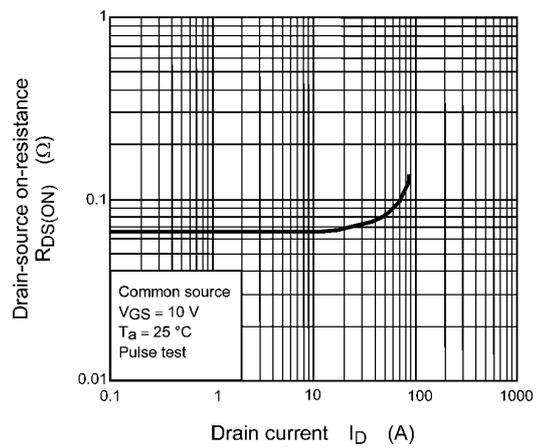
**Fig. 8.6  $R_{DS(ON)} - I_D$**
