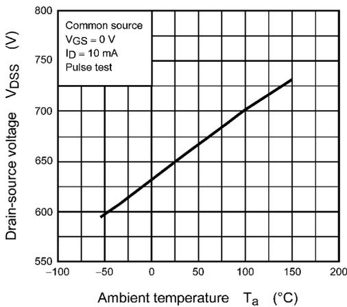
**Fig. 8.5  $V_{DS} - T_a$**
