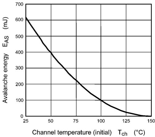
**Fig. 8.14  $E_{AS} - T_{ch}$**
