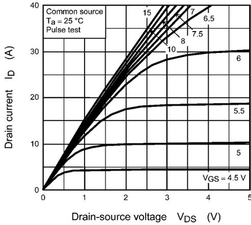
**Fig. 8.1  $I_D - V_{DS}$**
