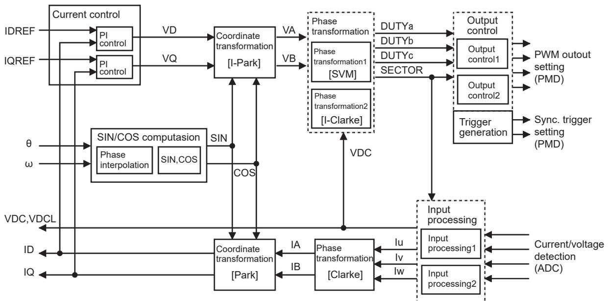
Figure 15-1 Block Diagram of Vector Control
