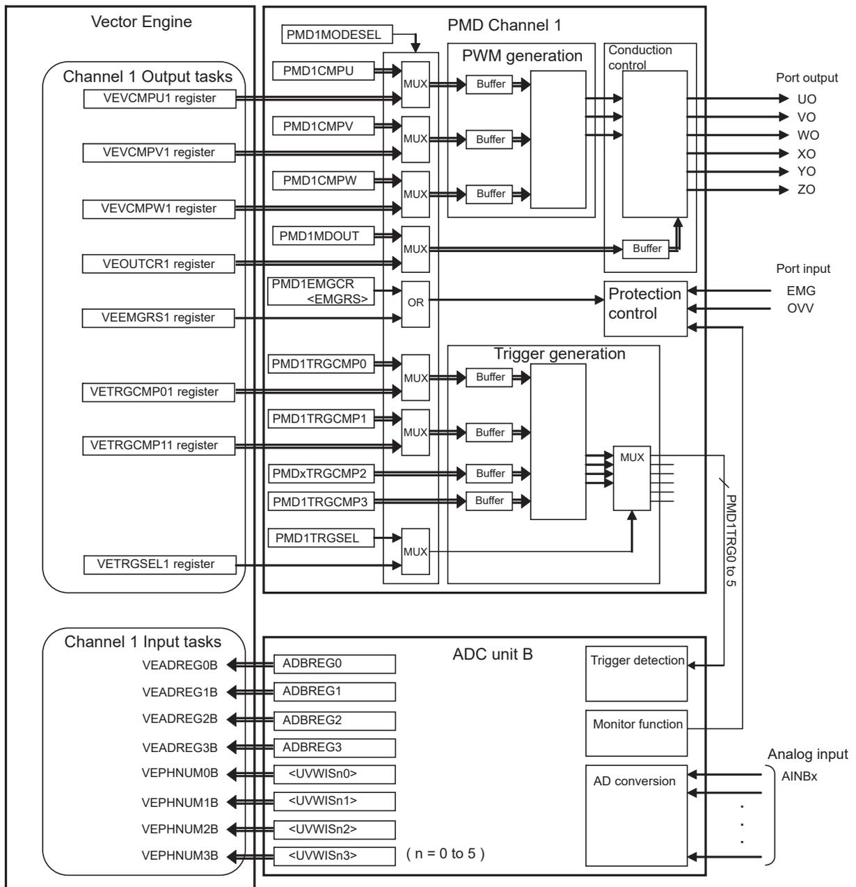
Figure 15-3 Interaction among Vector Engine, PMD and ADC
