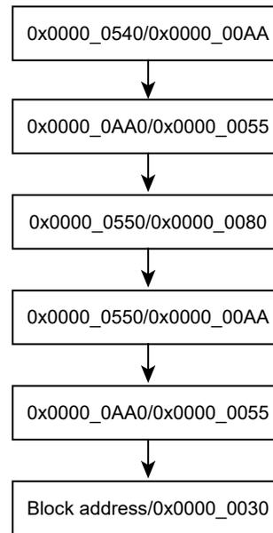
Figure 22-5 Flowchart of automatic erase
