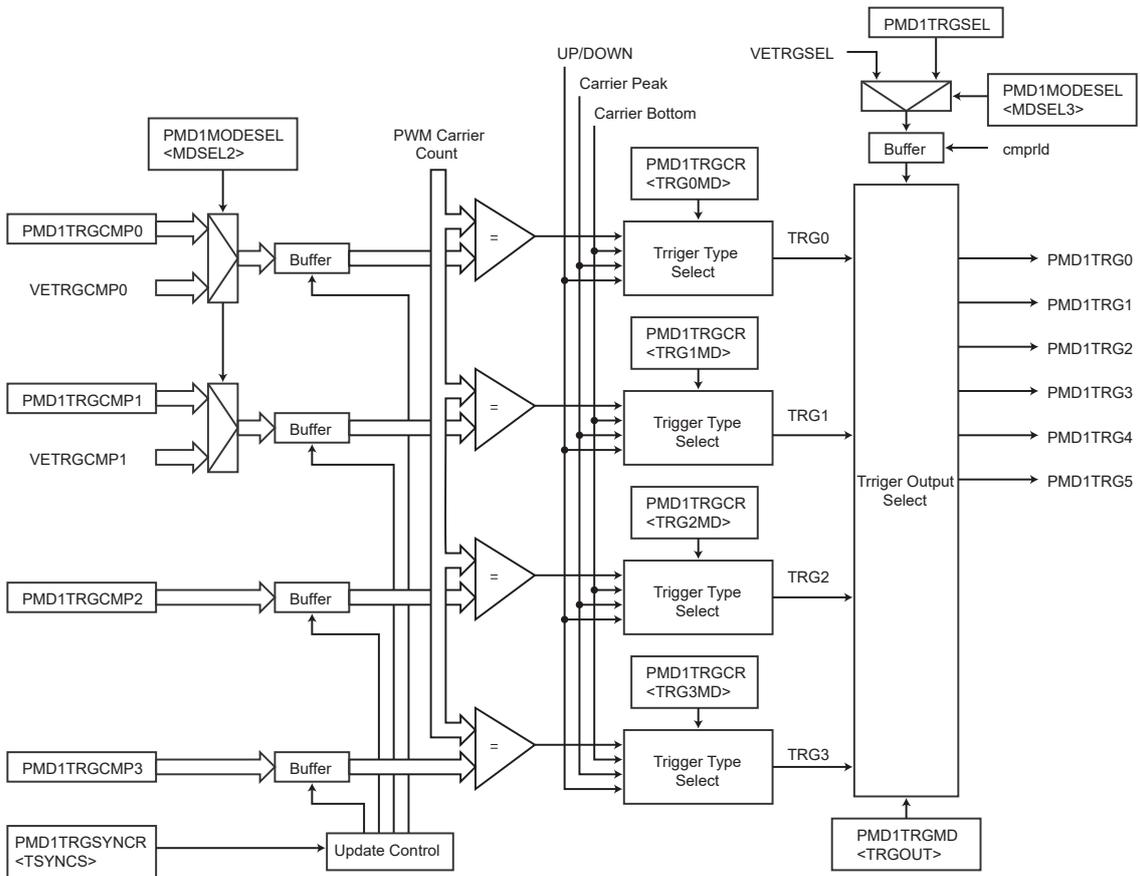
Figure 14-10 Sync Trigger Generation Circuit
