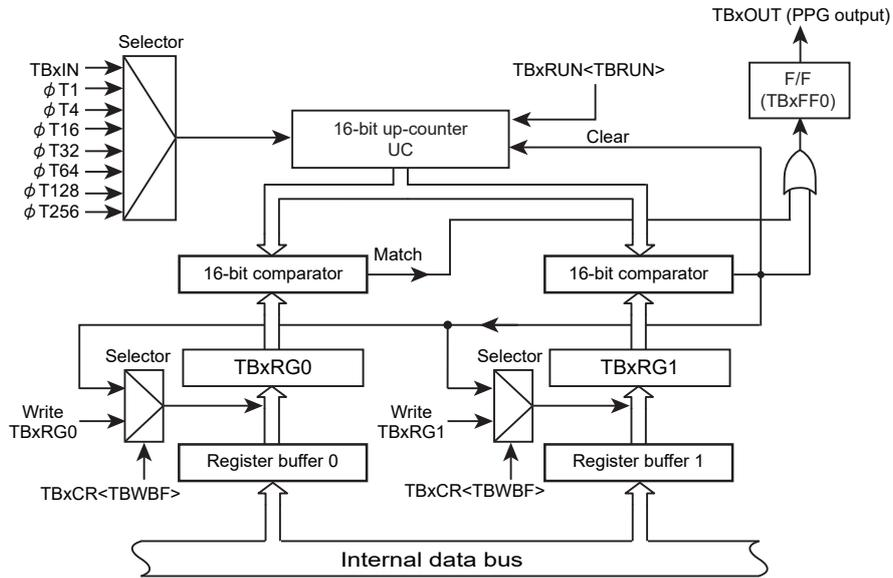
Figure 10-4 Block Diagram of 16-bit PPG Mode
