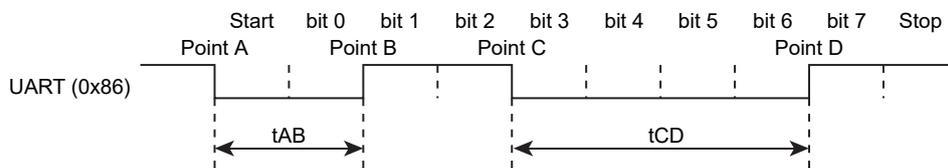
Figure 22-6 Serial operation mode determination data
