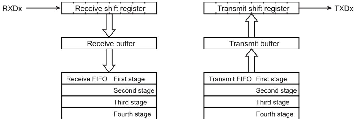
Figure 11-4 The Configuration of Buffer and FIFO
