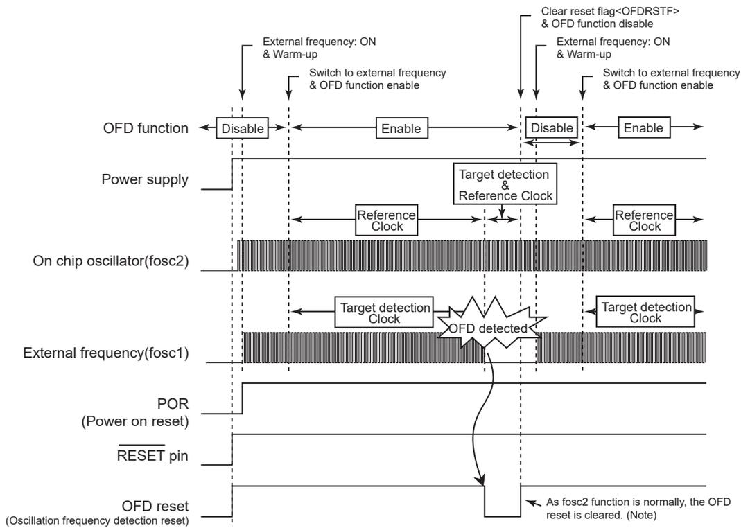
Note: The target clock is set without 10MHz into OFDMNPLLOFF and OFDMXPLLOFF. (eg, setting to 8MHz value to these registers) And when the target clock frequency is fosc1 and the reset generated by OFD, the reset might be generated continuously due to as abnormal detection until OFD detects correctly.
