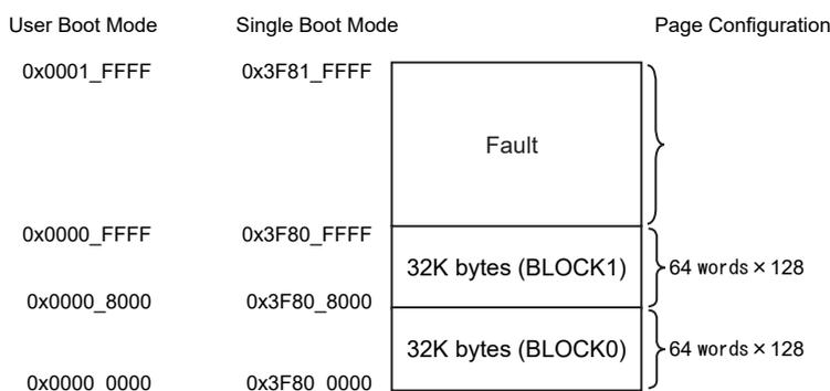
Figure 22-1 Block configuration
