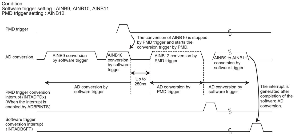
Figure 13-7 AD conversion by PMD trigger
