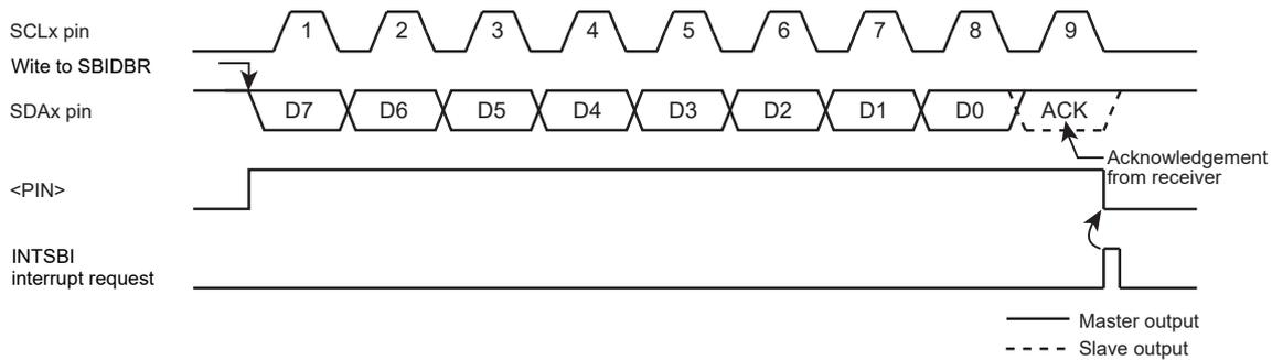
Figure 12-10 <BC[2:0]>= "000", <ACK>= "1" (Transmitter Mode)
