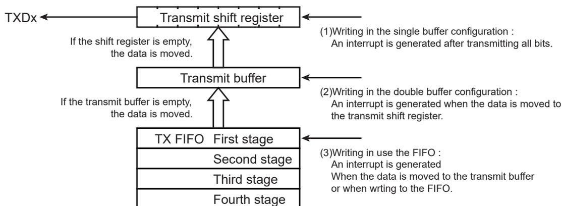
Figure 11-14 Transmit Buffer / FIFO Configuration Diagram
