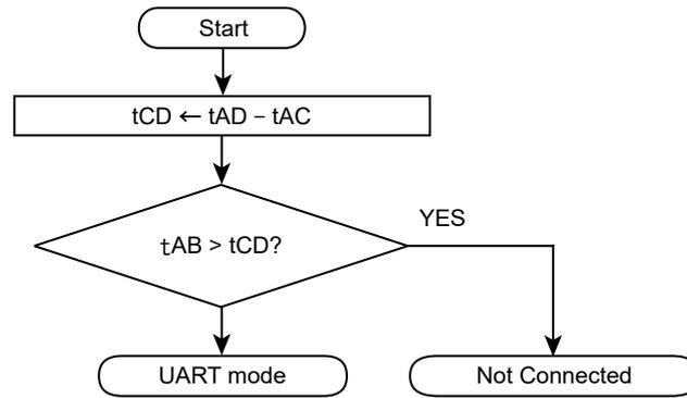
Figure 22-8 Serial operation mode determination flowchart
