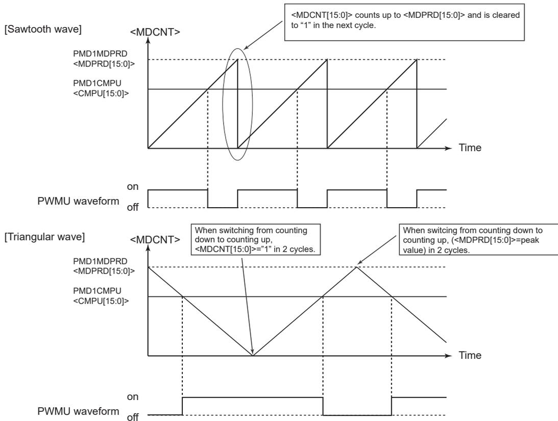
Figure 14-5 PWM Waveforms
