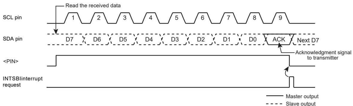
Figure 12-11 <BC[2:0]>= "000", <ACK>= "1" (Receiver Mode)
