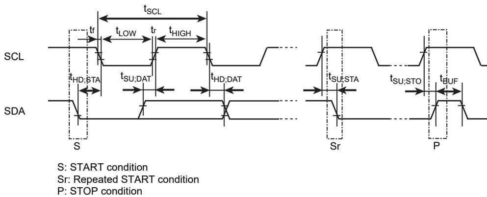
Figure 25-2 Serial Bus timing (I2C)
