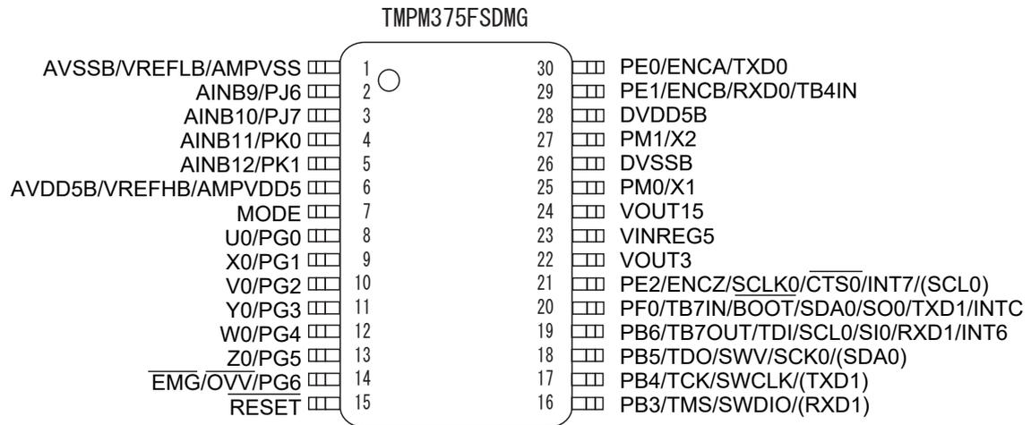
Figure 1-2 Pin Layout (SSOP30)
