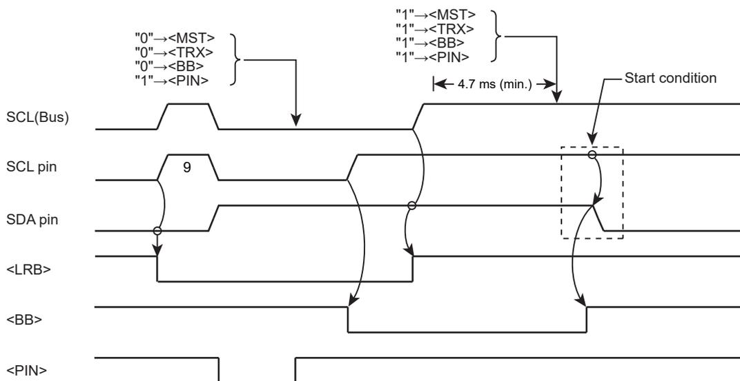
Figure 12-14 Timing Chart of Generating a Restart
