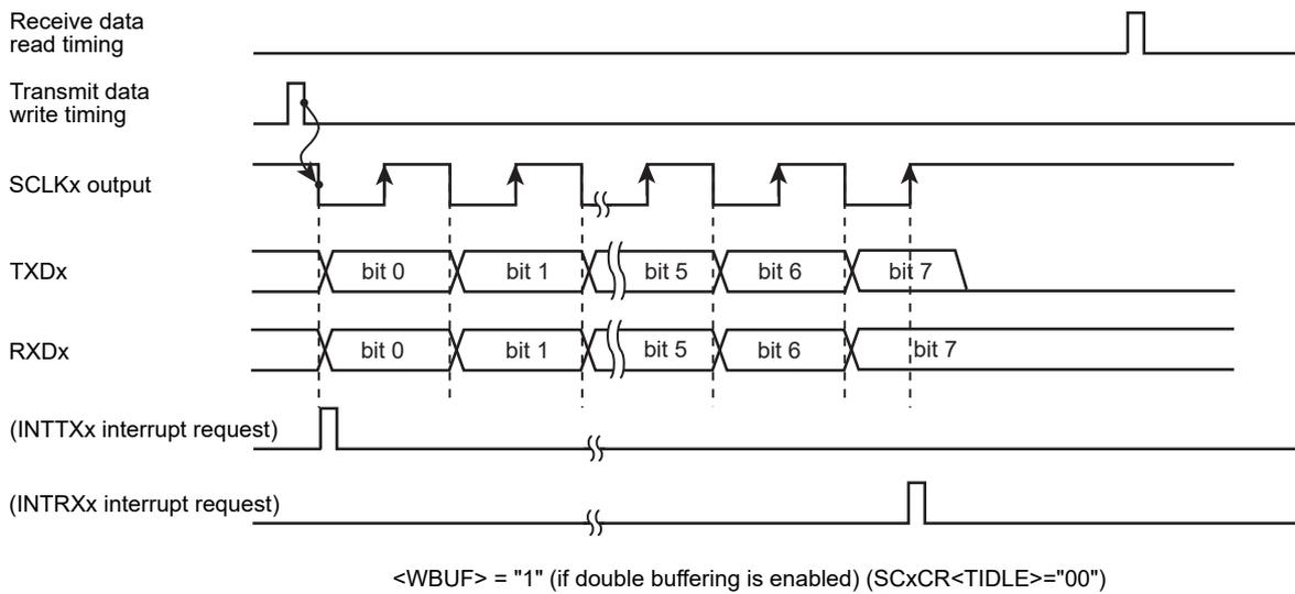
Figure 11-19 Transmit/Receive Operation in the I/O Interface Mode (SCLK Output Mode)
