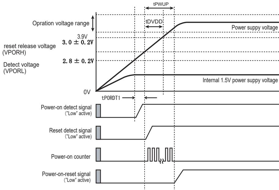
Figure 18-2 Power-on-reset operation timing
