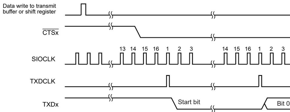
Figure 11-12  $\overline{CTSx}$  Signal timing
