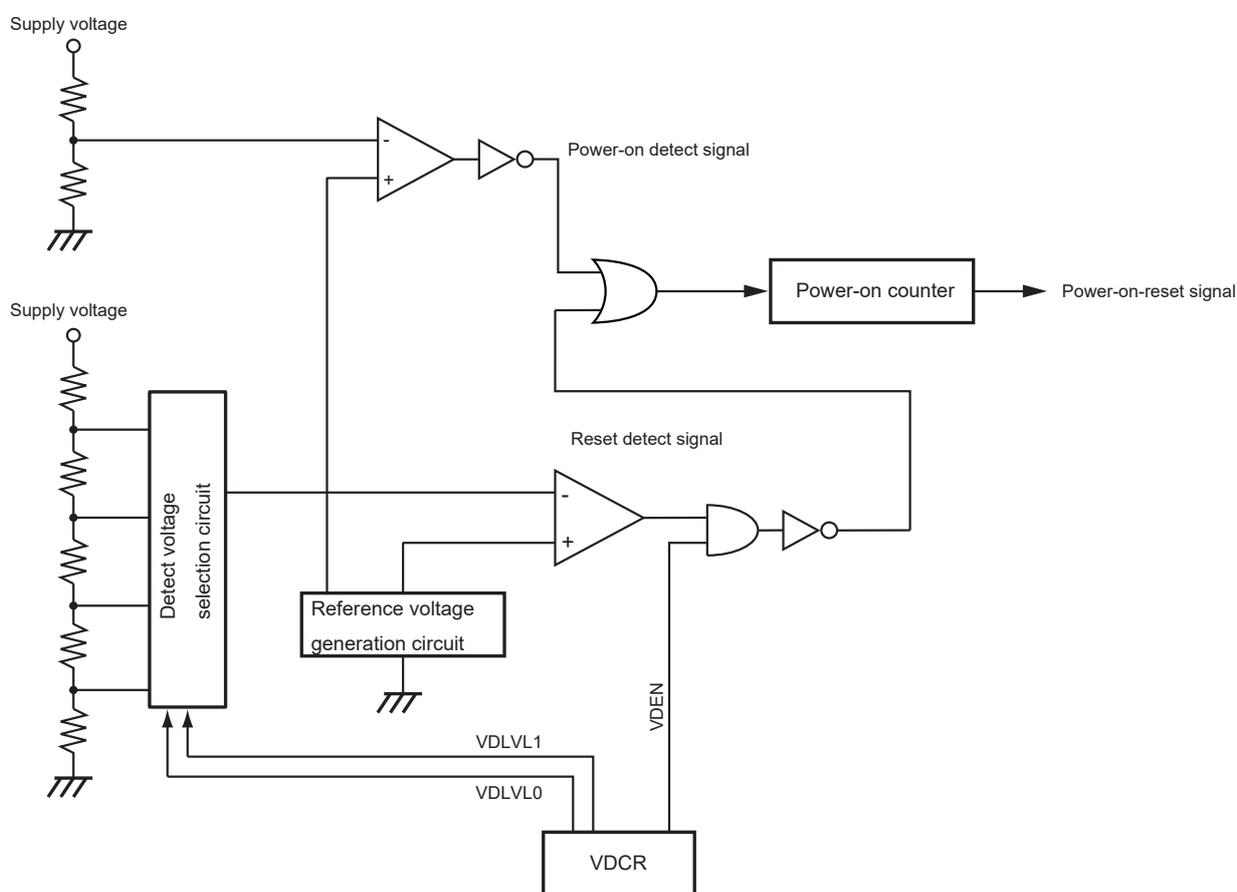
Figure 18-1 Power-on-reset circuit
