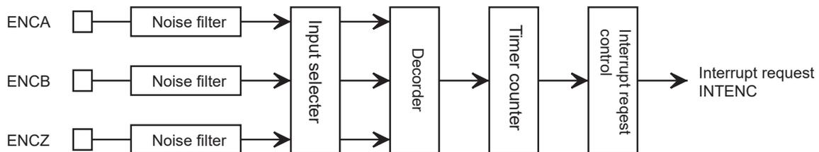
Figure 17-1 Block diagram of encoder input circuit
