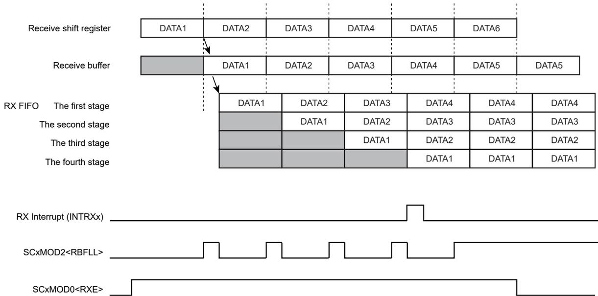
Figure 11-6 Receive FIFO Operation
