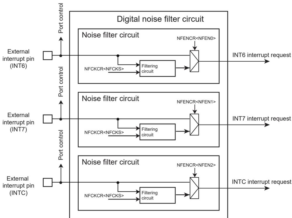
Figure 8-1 Circuit diagram of digital noise filter
