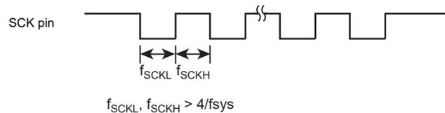
Figure 12-16 Maximum Transfer Frequency of External Clock Input
