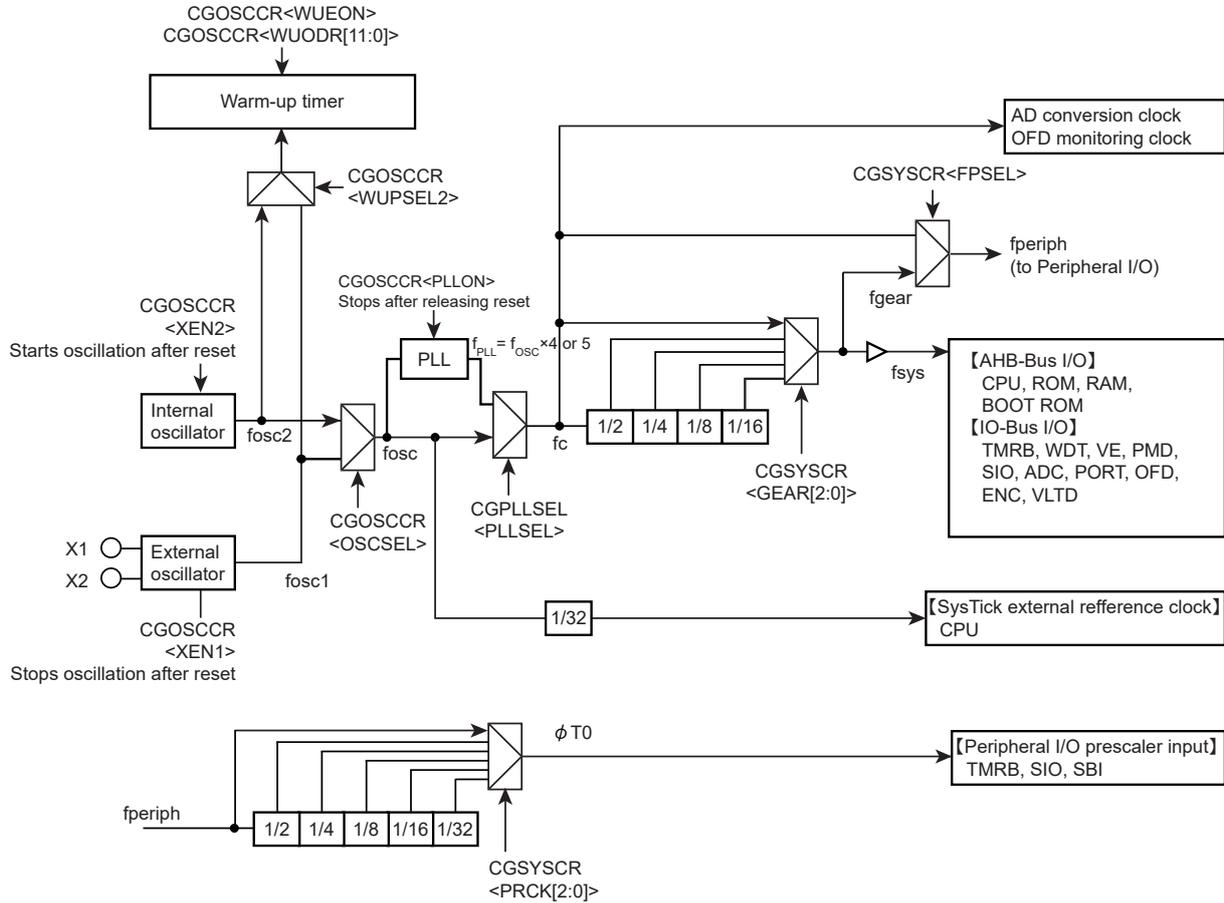
Figure 5-1 Clock Block Diagram
