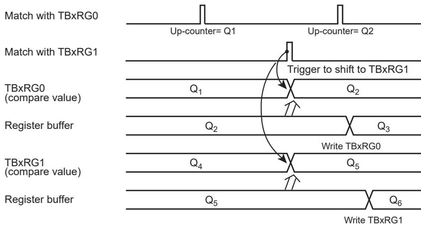
Figure 10-3 Register Buffer Operation
