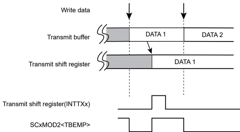
Figure 11-8 Operation of Transmission Buffer (Double-buffer is enabled)
