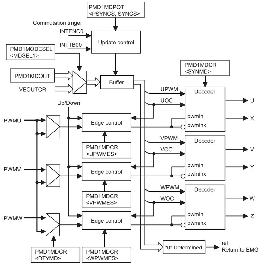
Figure 14-7 Conduction Control Circuit
