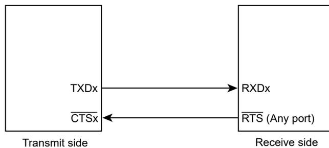
Figure 11-11 Handshake Function
