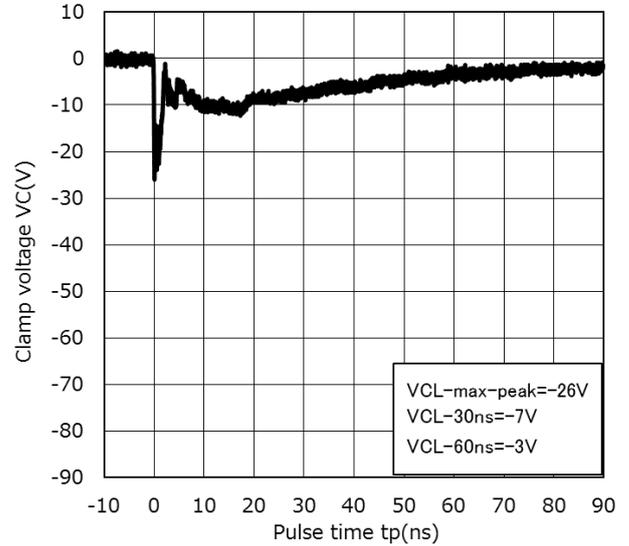
Clamp Waveform -8 kV (Note 3)
