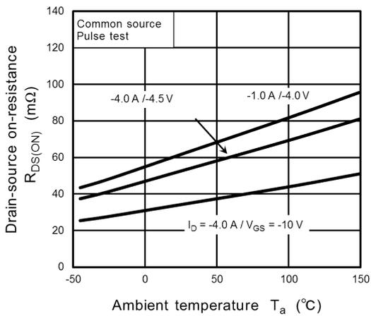
Fig. 7.5  $R_{DS(ON)} - T_a$
