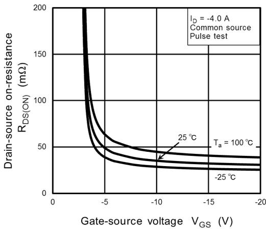
Fig. 7.3  $R_{DS(ON)} - V_{GS}$
