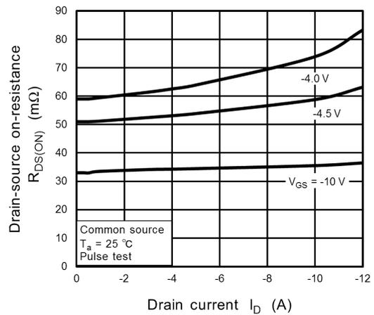
Fig. 7.4  $R_{DS(ON)} - I_D$
