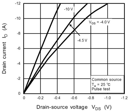
Fig. 7.1  $I_D - V_{DS}$
