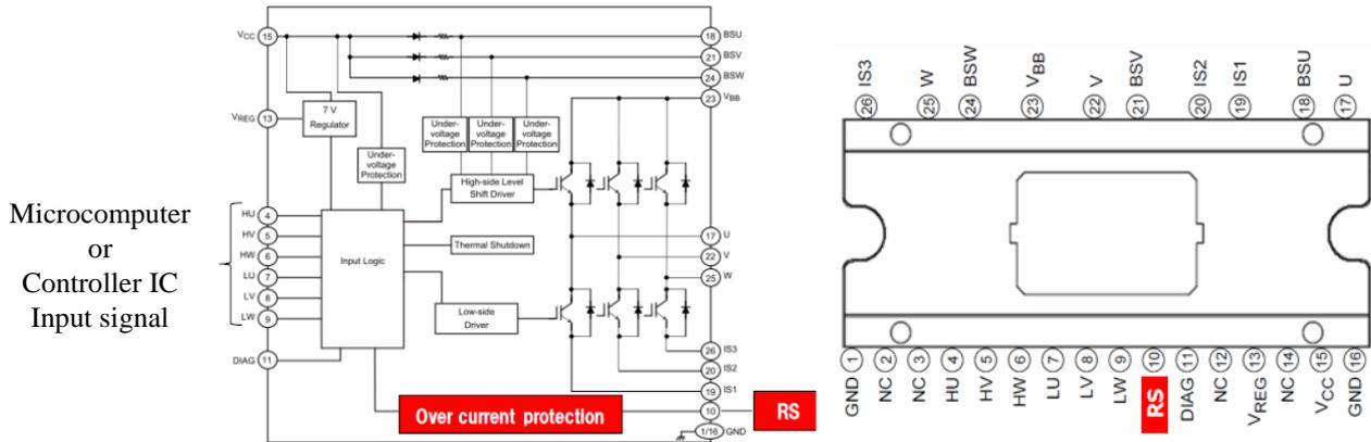
Figure 1-3 TPD4123K/TPD4144K/TPD4135K Block diagram and pin assignment
