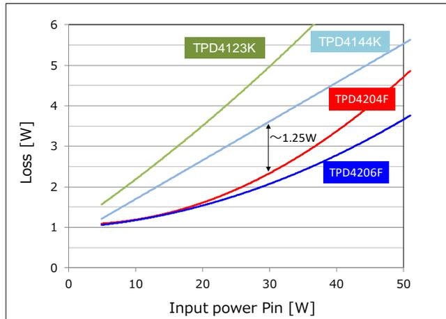
Figure 4-1 Loss-Input power Curve
