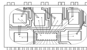
**Figure 1-2 Internal Structural Diagram: SSOP30**
