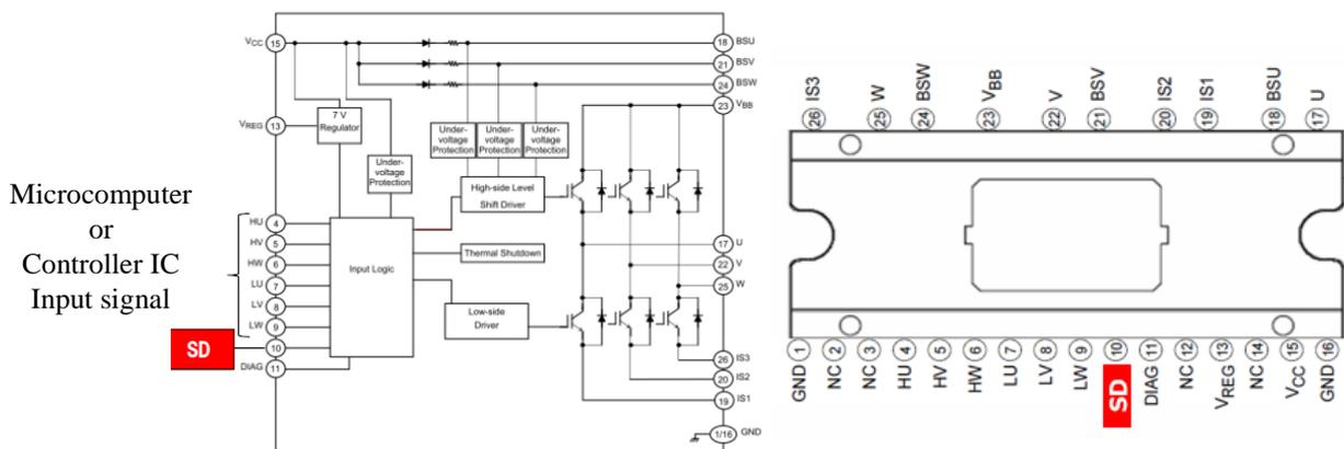
Figure 1-4 TPD4123AK/TPD4144AK/TPD4135AK Block diagram and pin assignment
