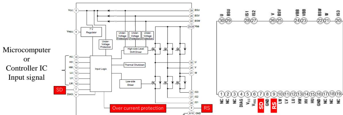
Figure 1-5 TPD4204F/TPD4206F/TPD4207F Block diagram and pin assignment
