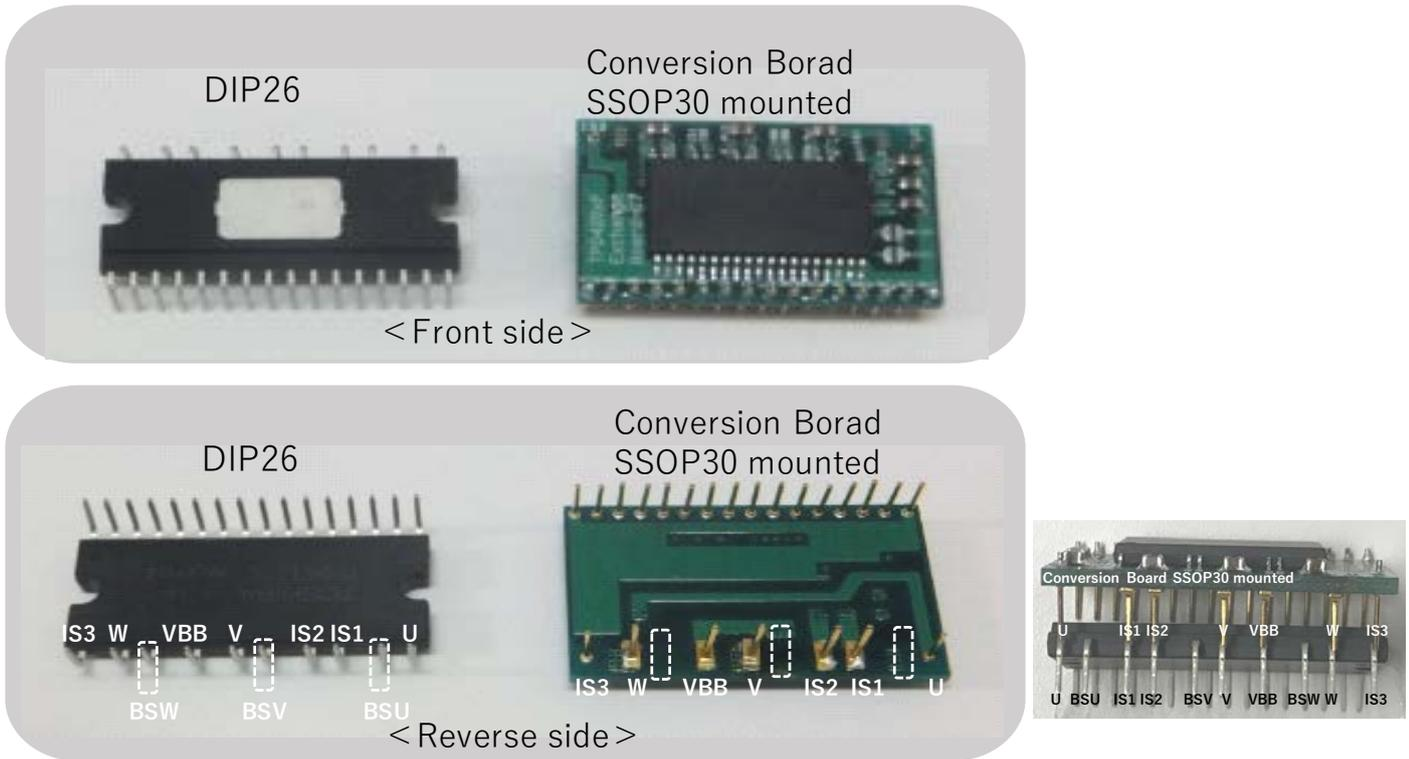
SSOP30 can be evaluated by inserting and soldering a conversion board with a SSOP30 into an existing board designed for DIP26.
