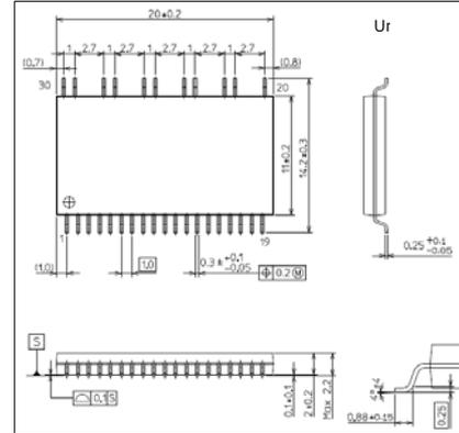
Figure 2-2 SSOP30 Dimensions
