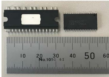
Figure 2-3 Comparing DIP26 and SSOP30
