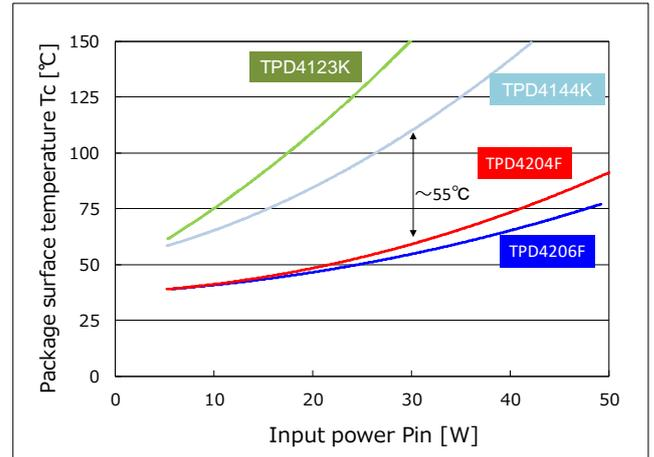
Figure 4-2 Package Surface Temperature-Input Power Curve
