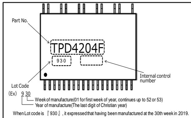
Figure 2-4 SSOP30 Marking
