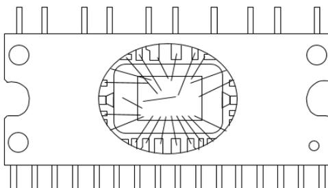
**Figure 1-1 Internal Structural Diagram: DIP26**
