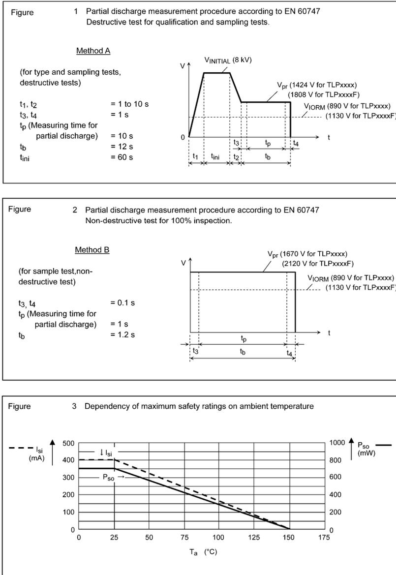
Fig. 17.3 Measurement Procedure
