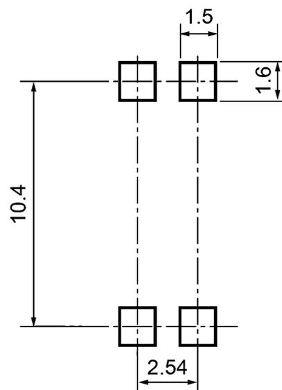
Fig. 16.2 Lead forming and taping option (LF4), (TP4)
