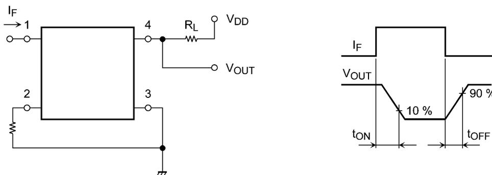
Fig. 13.1 Switching Time Test Circuit and Waveform
