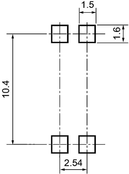
Fig. 18.2 Lead forming and taping option (LF4), (TP4)
