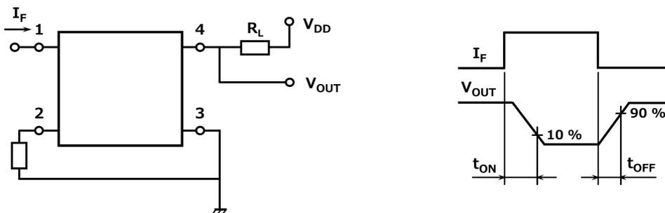
Fig. 15.1 Switching Time Test Circuit and Waveform
