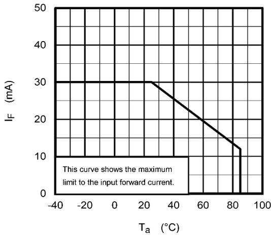
Fig. 16.1 I<sub>F</sub> - T<sub>a</sub>
