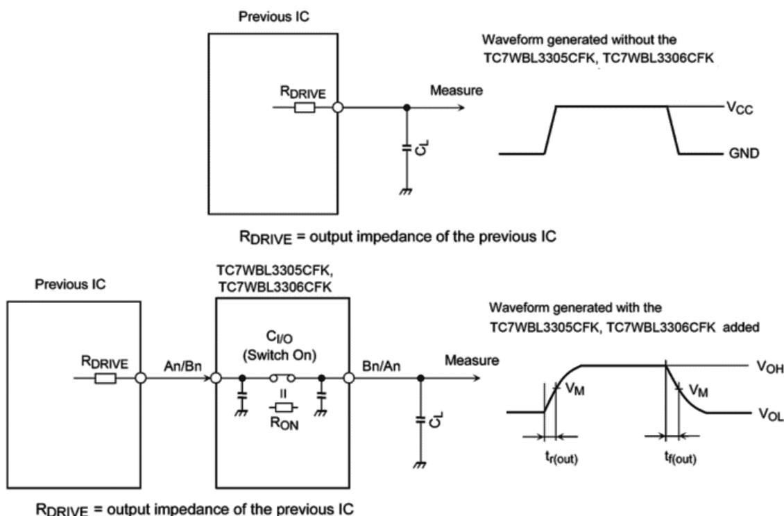
Fig. 12.1 Calculation Circuit
