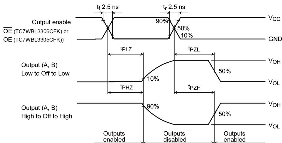
Fig. 11.6.2 AC Waveform  $t_{PLZ}, t_{PHZ}, t_{PZL}, t_{PZH}$
