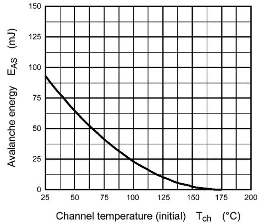
**Fig. 8.14**  $E_{AS} - T_{ch}$
