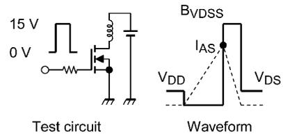
$$R_G = 25 \Omega, V_{DD} = 80 \text{ V}, L = 24 \mu\text{H} \quad E_{AS} = \frac{1}{2} \cdot L \cdot I_{AS}^2 \cdot \left( \frac{B_{VDSS}}{B_{VDSS} - V_{DD}} \right)$$
