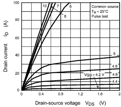
**Fig. 8.2**  $I_D - V_{DS}$
