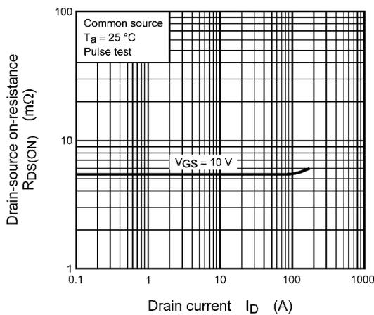
**Fig. 8.5**  $R_{DS(ON)} - I_D$
