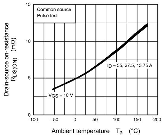
**Fig. 8.6**  $R_{DS(ON)} - T_a$
