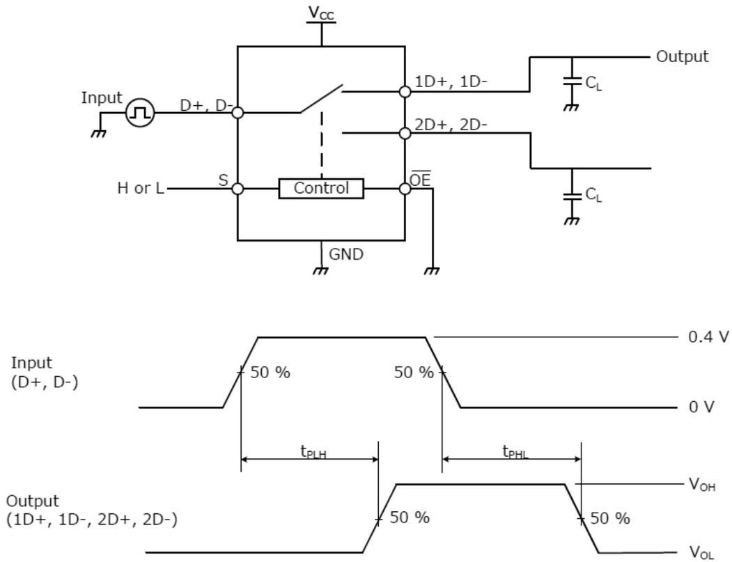
Fig. 11.1 Propagation Delay Time ( $t_{PLH}$ ,  $t_{PHL}$ )
