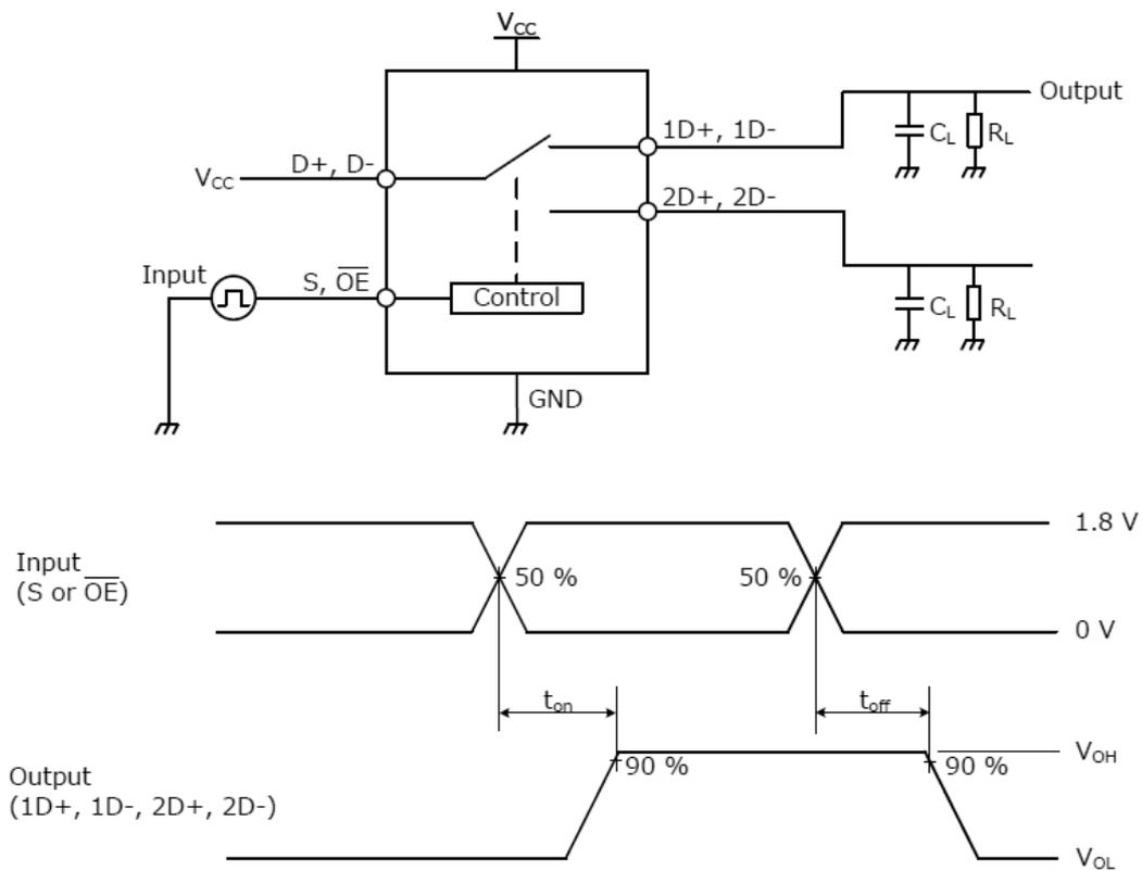
Fig. 11.2 Turn-ON and Turn-OFF Times ( $t_{on}$ ,  $t_{off}$ )
