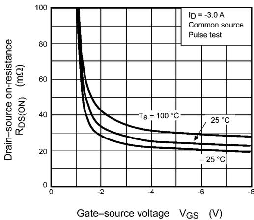
Fig. 7.3  $R_{DS(ON)} - V_{GS}$
