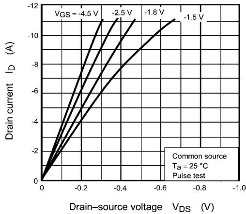
Fig. 7.1  $I_D - V_{DS}$
