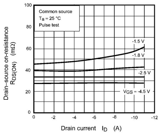
Fig. 7.4  $R_{DS(ON)} - I_D$
