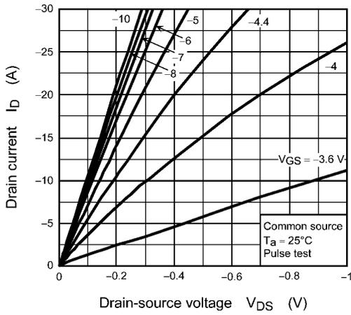
Fig. 8.1  $I_D - V_{DS}$
