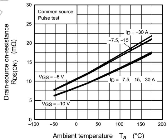
Fig. 8.6  $R_{DS(ON)} - T_a$
