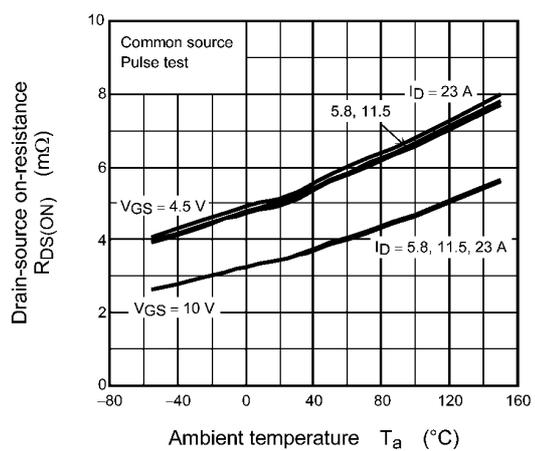
Fig. 8.6  $R_{DS(ON)} - T_a$
