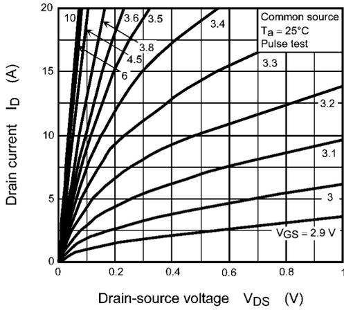
Fig. 8.1  $I_D - V_{DS}$
