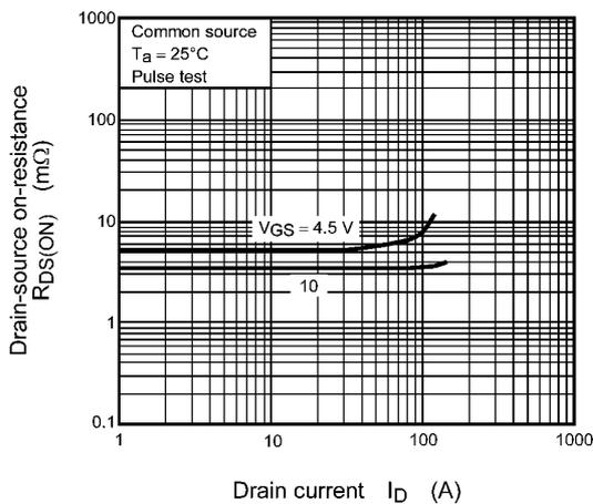
Fig. 8.5  $R_{DS(ON)} - I_D$
