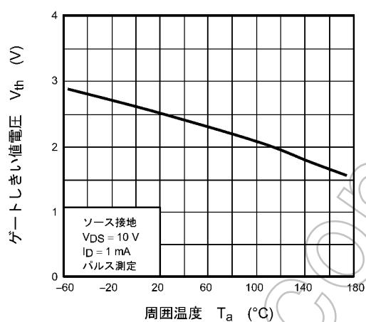
図 8.9  $V_{th}$  -  $T_a$  (注7)
