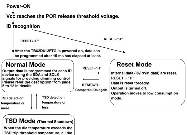
outputs are disabled, while internal data is retained.
