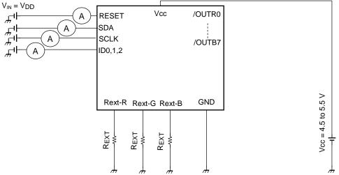
Test Circuit 2: Low-Level Input Current (IIL)
