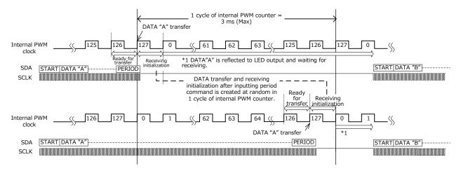
In case of matching asynchronously the timing between SCLK end and internal data update, the start command at the beginning of next pattern may not be received. That may occur in the pattern of first IC if there are patterns for two or more ICs. That does not occur if the pattern length is as follows.
