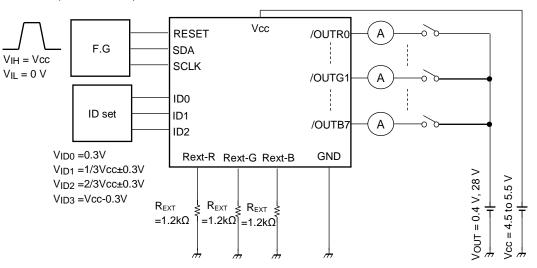
Test Circuit 5: Switching Characteristics
