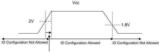
Care should be taken during the period between the POR released timing and the timing when power supply has reached the rated Vcc voltage.
