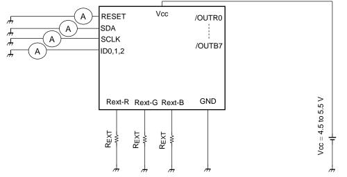
Test Circuit 3: Supply Current
