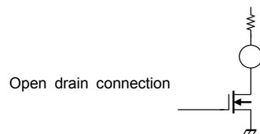
The rest voltage of the  $\overline{MO}$  (output terminal) becomes 0.5 V(max.) when  $I_O$  is 1 mA.
