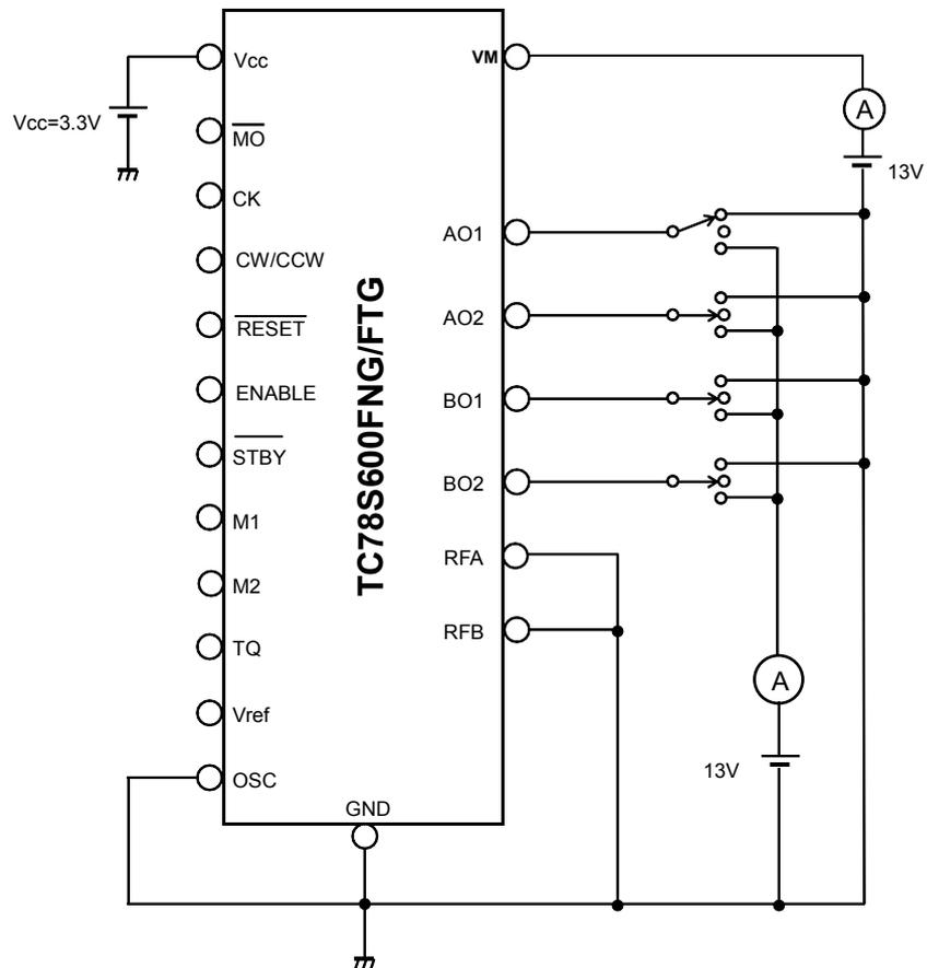
**AC electric characteristics Test points 7: CK(OSC)-OUT**
