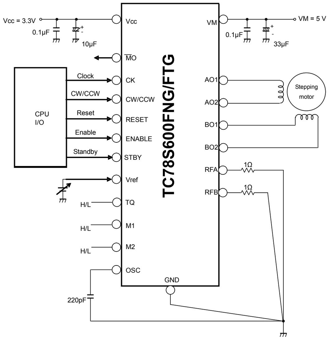
Note 1: Capacitors for the power supply lines should be connected as close to the IC as possible.
