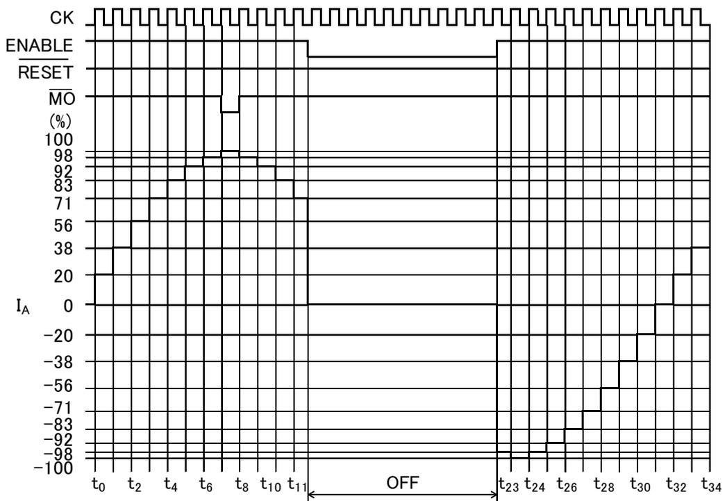
**Relationship between the  $\overline{\text{RESET}}$  Input and the Phase Current and  $\overline{\text{MO}}$  Outputs**
