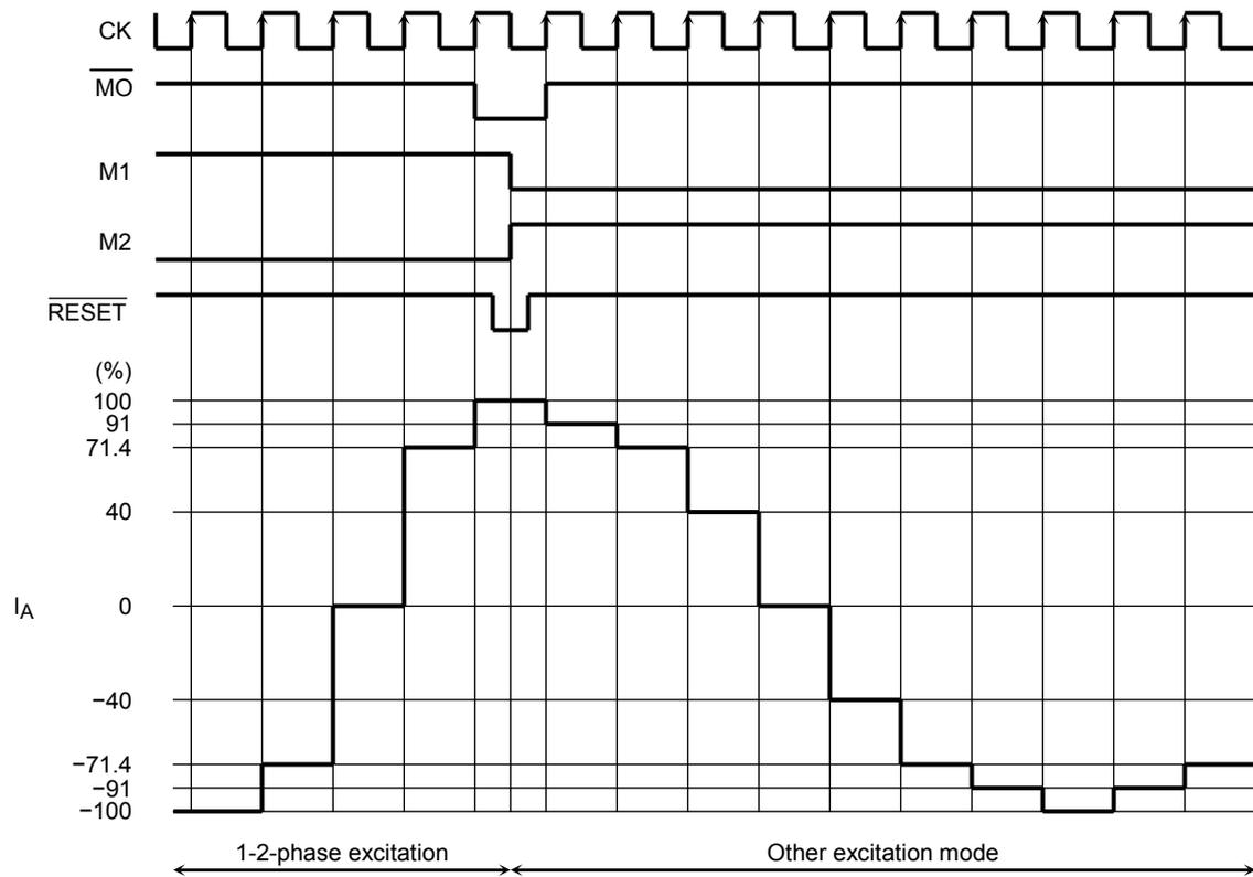
M1 and M2 should be changed after  $\overline{\text{RESET}}$  is set low in the initial state ( $\overline{\text{MO}} = \text{Low}$ ). Smooth current waveform cannot be gained if they are changed without setting  $\overline{\text{RESET}}$  low though  $\overline{\text{MO}}$  is set low.
