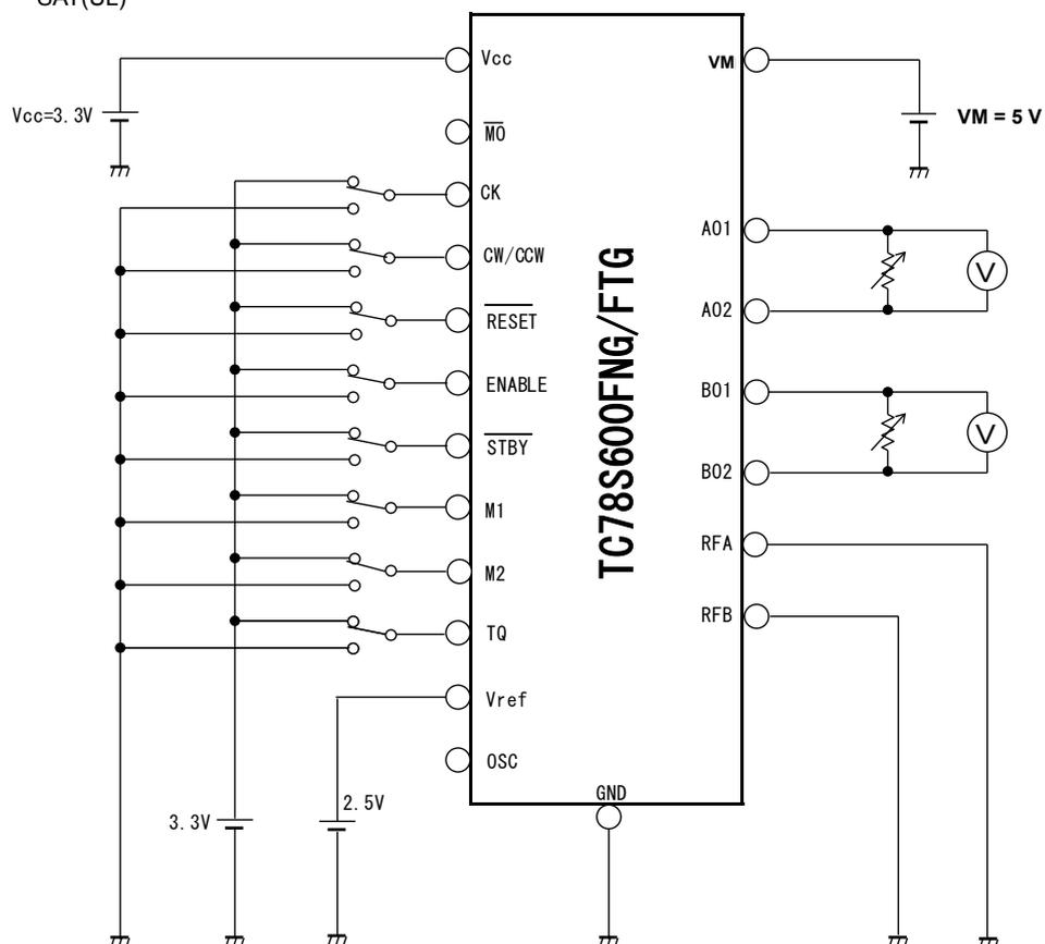
**Test circuit 5:**  $V_{FU}$ ,  $V_{FL}$
