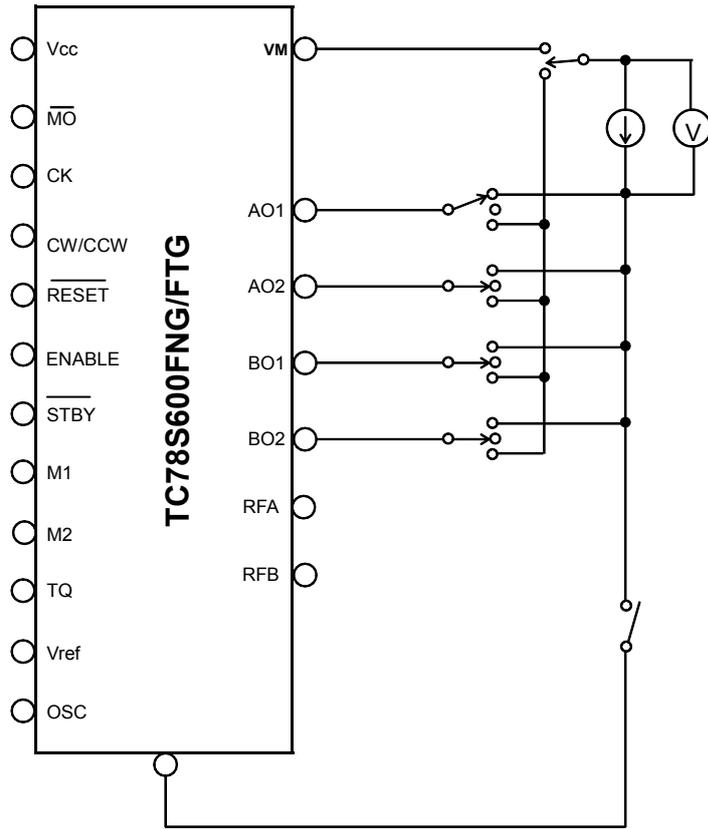
**Test circuit 6:**  $I_{OH}$ ,  $I_{OL}$
