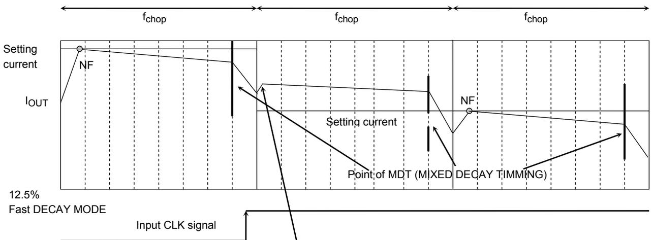
It is charged for a short time for current confirmation though the current is higher than the setting current.
