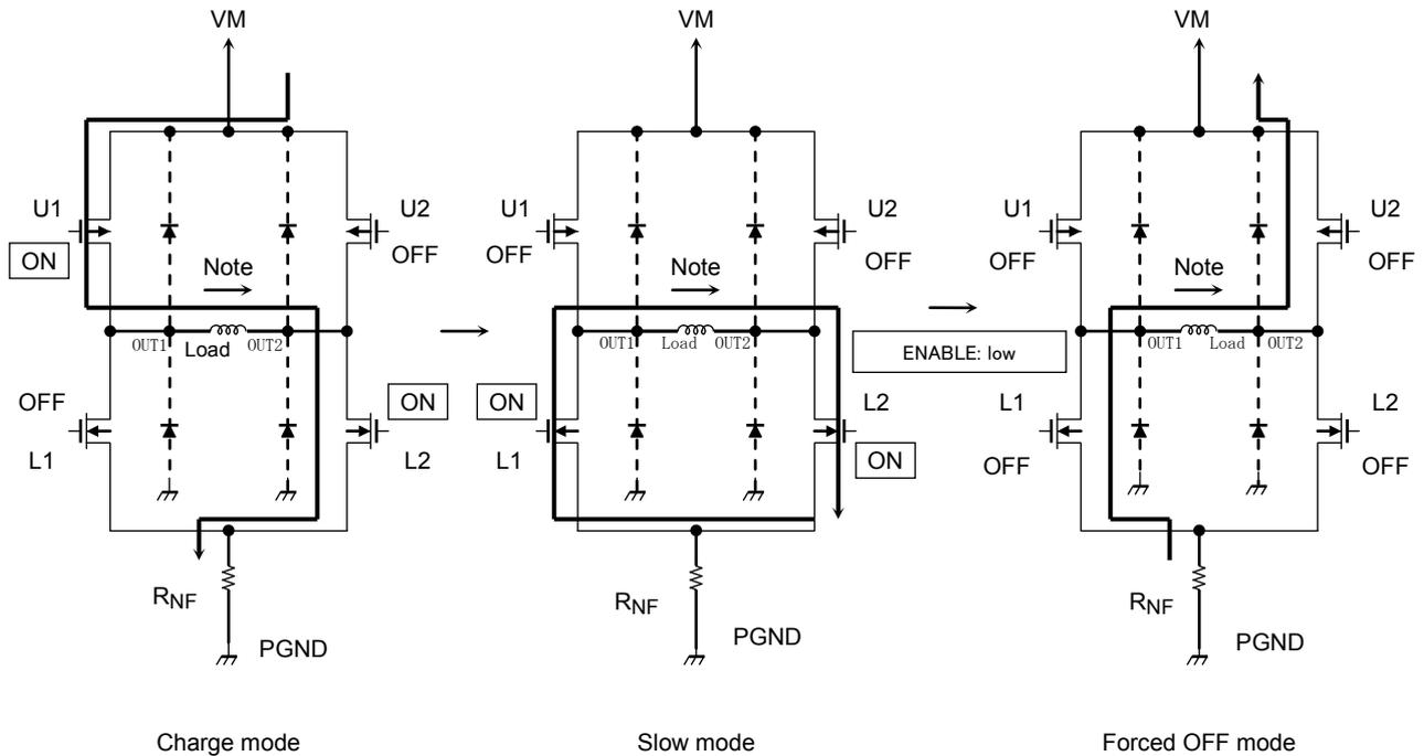
Parasitic diodes exist in the output transistors as shown above.
