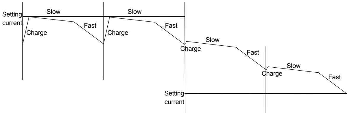
In MIXED DECAY MODE and FAST DECAY MODE, when output current is higher than setting current, CHARGE MODE does not exist (in a narrow sense, CHARGE MODE is very short time for detecting current) at the next chopping cycle. And it moves to SLOW and FAST MODE. SLOW MODE is moved to FAST MODE by MDT.
