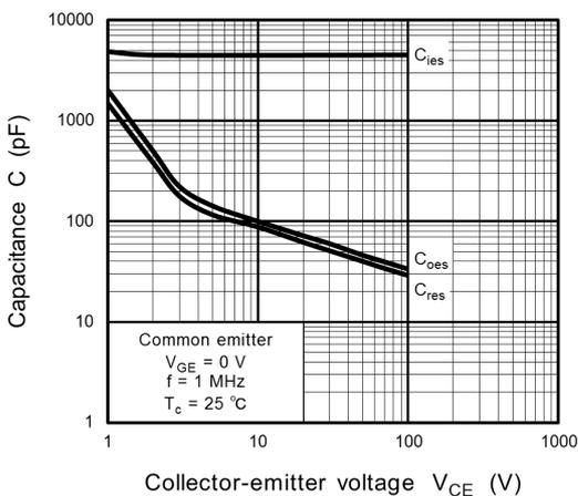
**Fig. 8.11 C -  $V_{CE}$**
