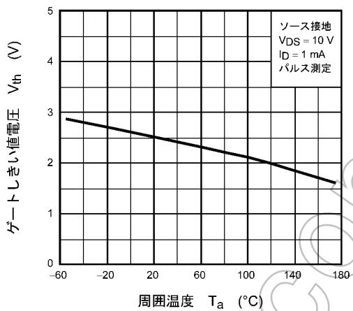
図 8.9  $V_{th}$  -  $T_a$  (注7)
