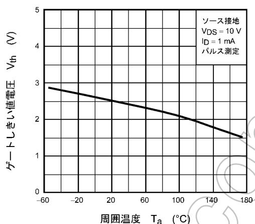
図 8.9  $V_{th}$  -  $T_a$  (注7)
