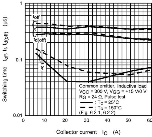
**Fig. 8.13**  $t_{off}$ ,  $t_r$ ,  $t_d(off)$  -  $I_C$
