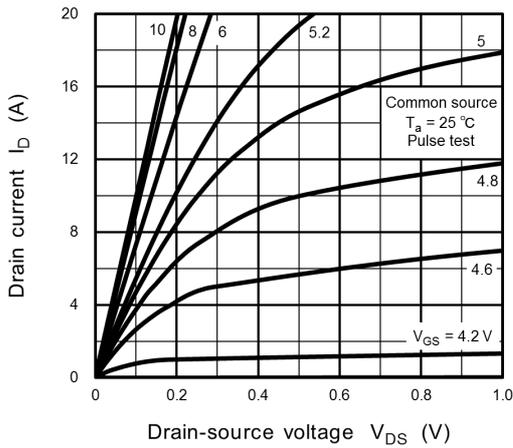
Fig. 8.1  $I_D - V_{DS}$
