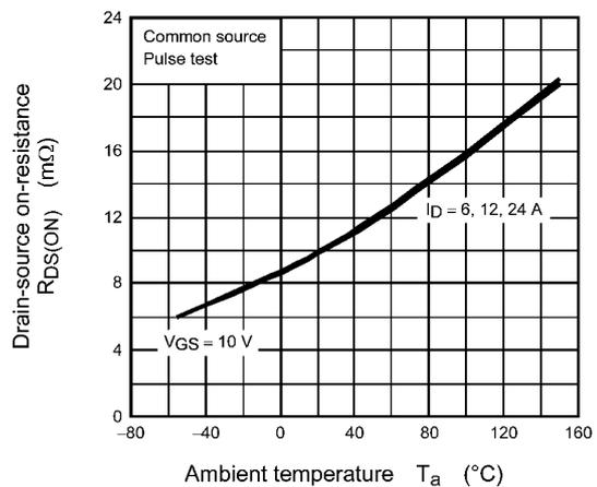
Fig. 8.6  $R_{DS(ON)} - T_a$
