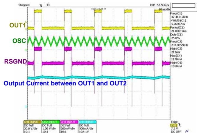
Reference waveforms when VREF = 2.0 V
