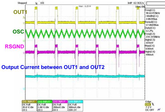
Reference waveforms when VREF = 0 V
