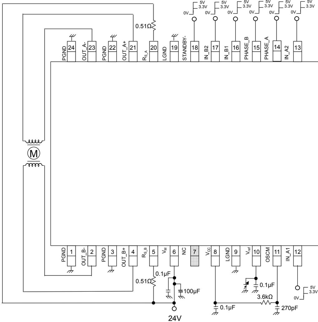
Note: I will recommend the addition of capacitor if necessary. The GND wiring must become one point as much as possible-earth.
