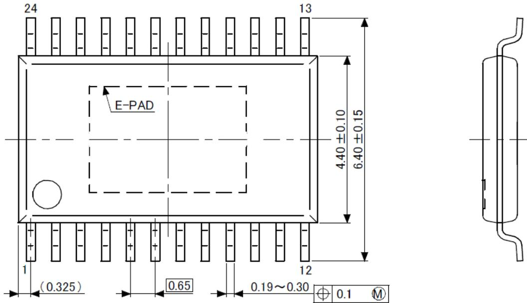
The heat sink is located on the back side and has dimensions of 2.85 mm × 4.05 mm.
