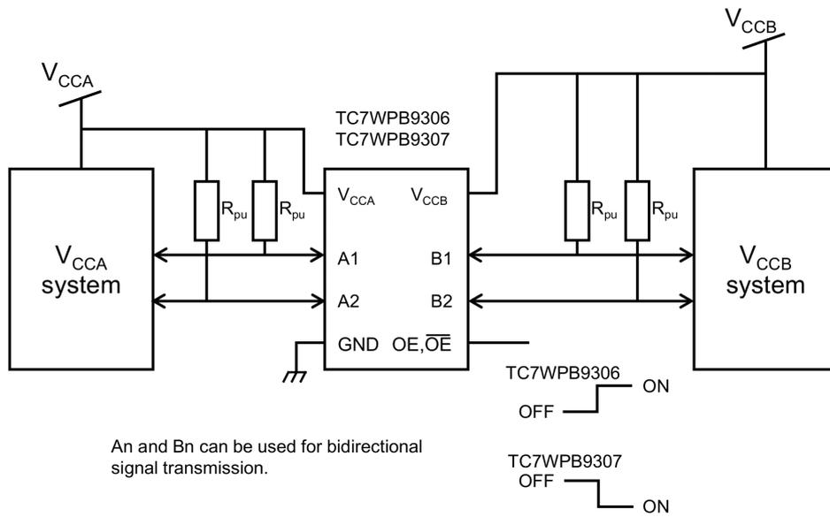
Note: The  $V_{CCA} < V_{CCB}$  voltage must be lower than the  $V_{CCB}$  voltage.
