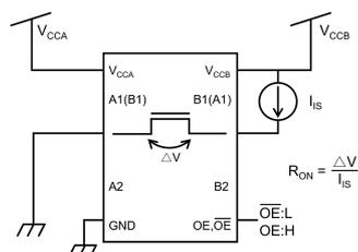
Fig. 12.1 ON-resistance Test Circuits
