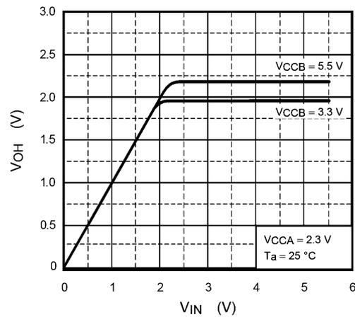
Fig. 15.3 Input/Output Characteristics (Typ.)
