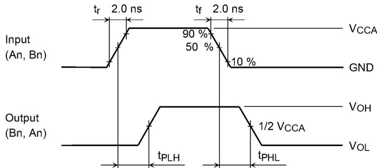
Fig. 13.3 AC Waveform of t<sub>PLH</sub>, t<sub>PHL</sub>
