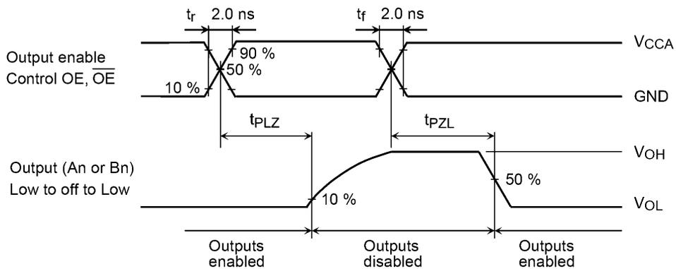
Fig. 13.4 AC Waveform of t<sub>PLZ</sub>, t<sub>PZL</sub>
