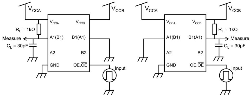
Fig. 13.2 t<sub>PLZ</sub>, t<sub>PZL</sub> Test Circuits
