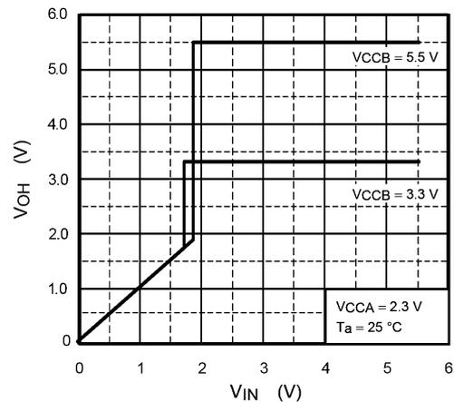
Fig. 14.3 Input/Output Characteristics (Typ.)
