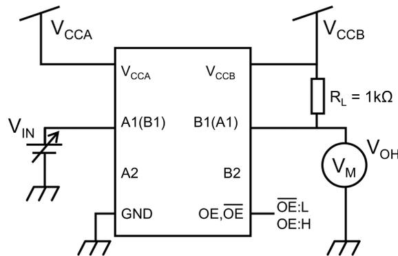
Fig. 14.1 Test Circuit
