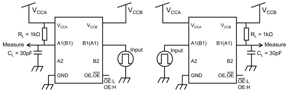
Fig. 13.1 t<sub>PLH</sub>, t<sub>PHL</sub> Test Circuits
