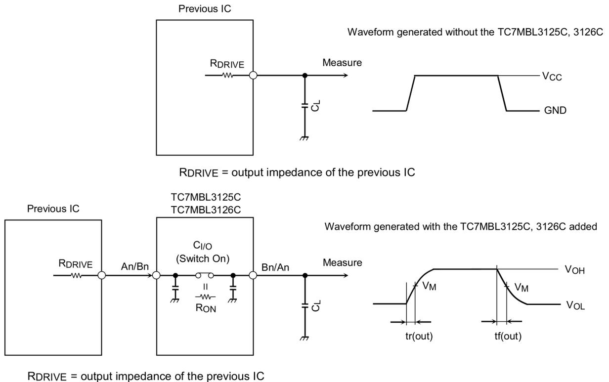
**Fig. 12.1 Calculation Circuit**
