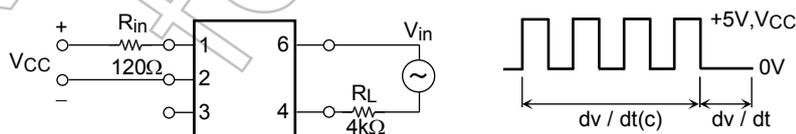
(Note 3): impulse noise durability test circuit
