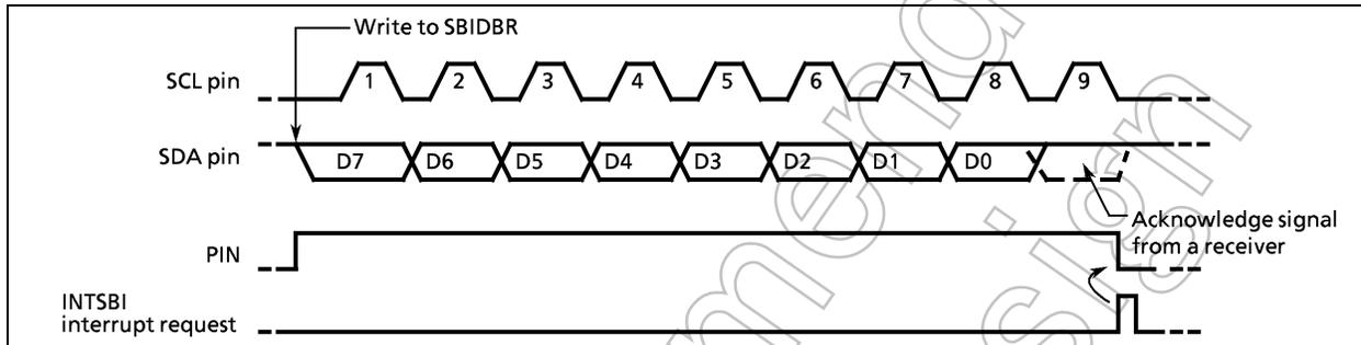
Figure 2-43. Example when BC = "000", ACK = "1" in Transmitter Mode
