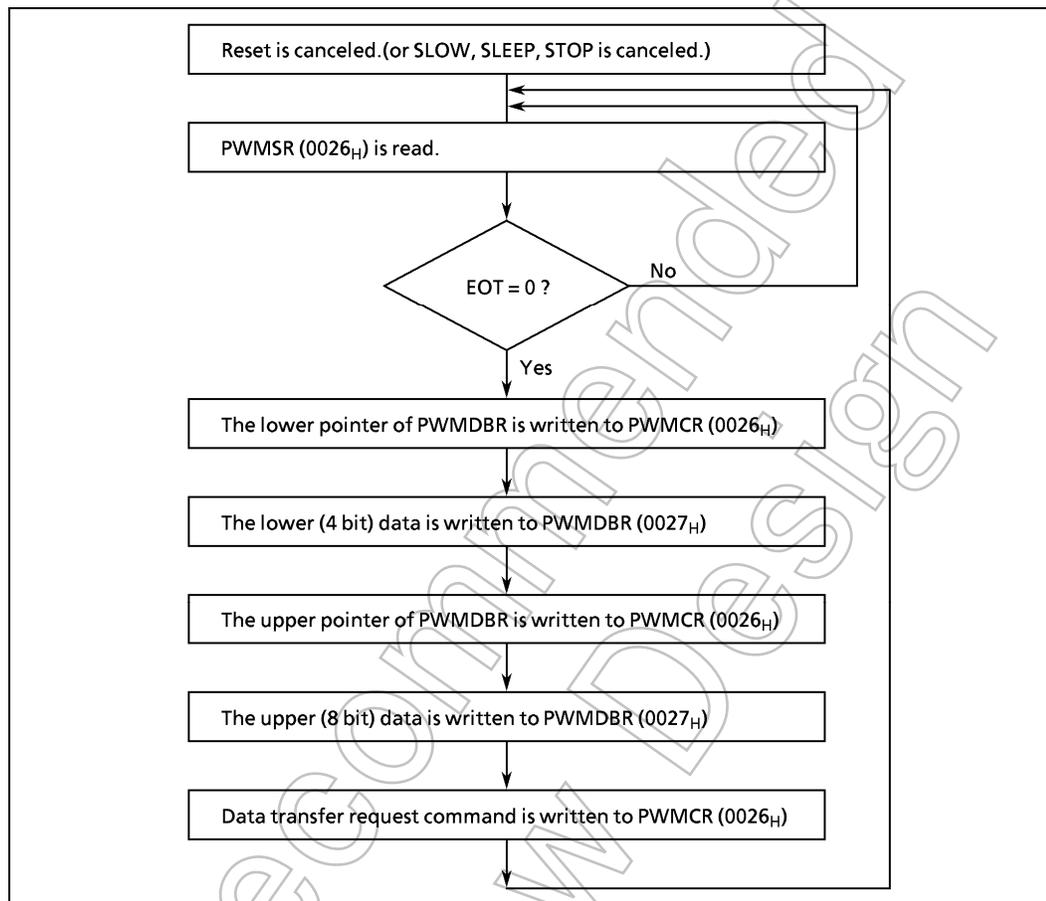
Figure 2-68 (2). Program Control Procedures for Channels
