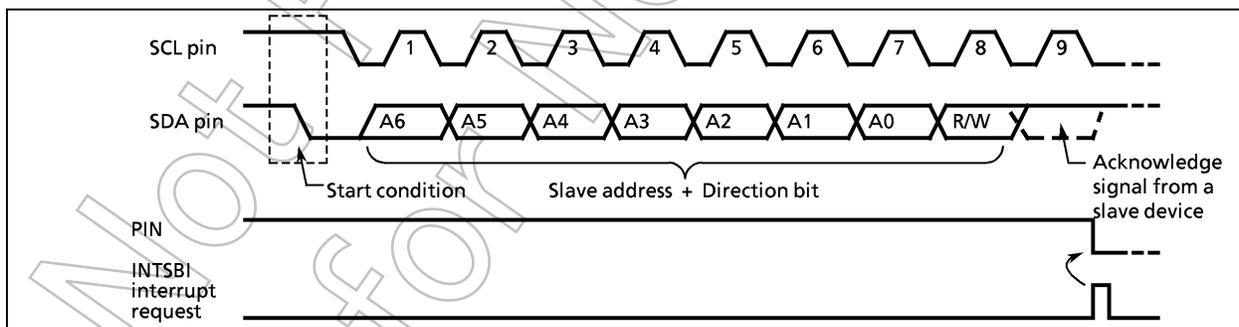
Figure 2-42. Start Condition Generation and Slave Address Transfer
