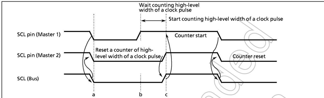
Figure 2-37. Clock Synchronization
