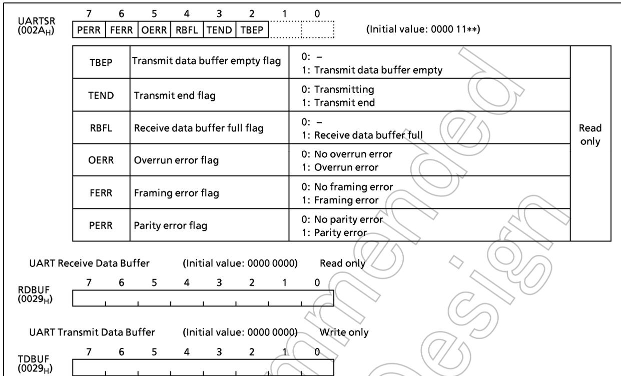
Figure 2-59. UART Status Register and Data Buffer Registers
