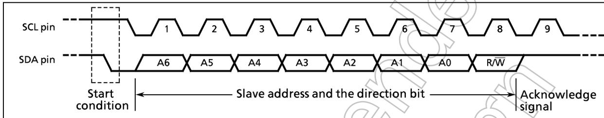
Figure 2-38. Start Condition Generation and Slave Address Generation
