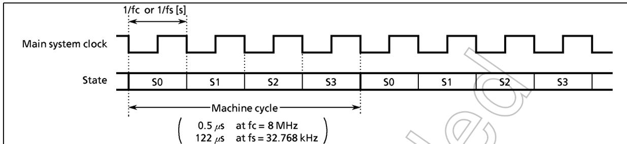
Figure 1-13. Machine Cycle
