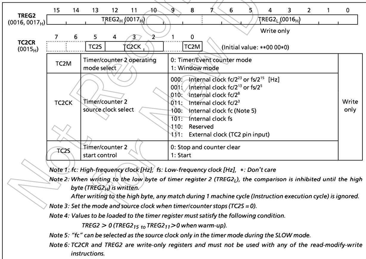
Figure 2-24. Timer Register 2 and TC2 Control Register
