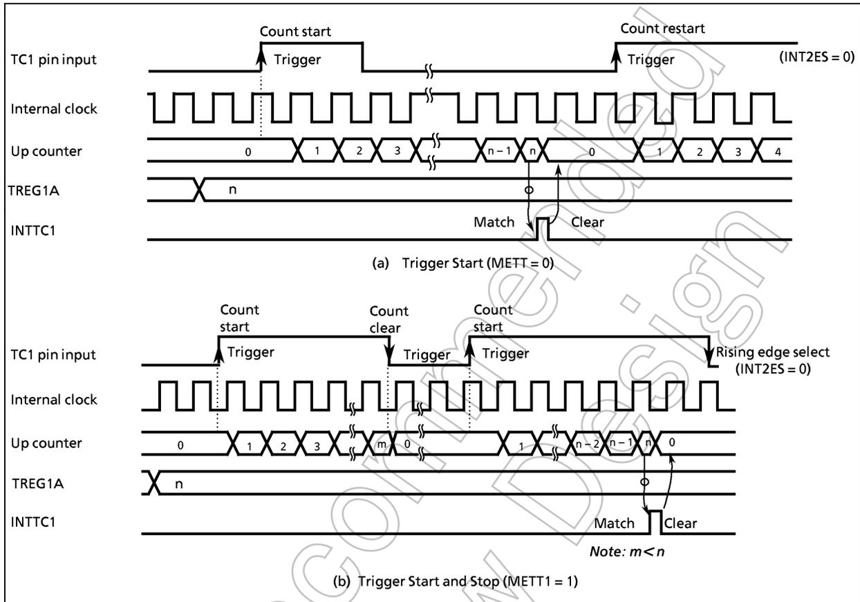
Figure 2-17. External Trigger Timer Mode Timing Chart
