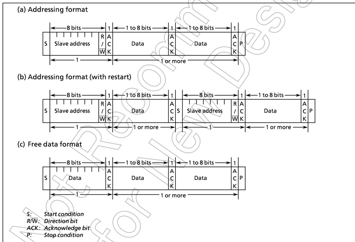
Figure 2-33. Data Format at I<sup>2</sup>C Bus Mode
