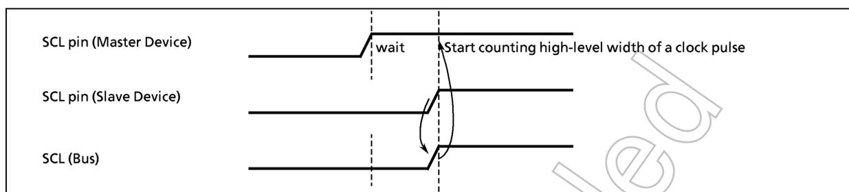
Figure 2-43. Clock Synchronization
