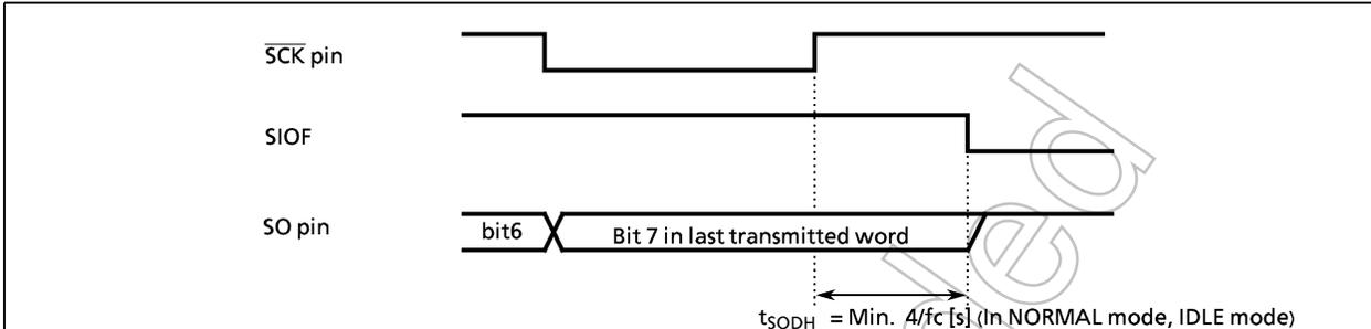
Figure 2-62. Transmitted Data Hold Time at End of Transmit / Receive
