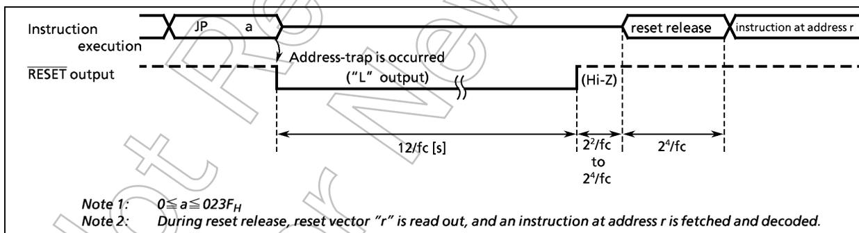
Figure 1-31. Address-Trap-Reset
