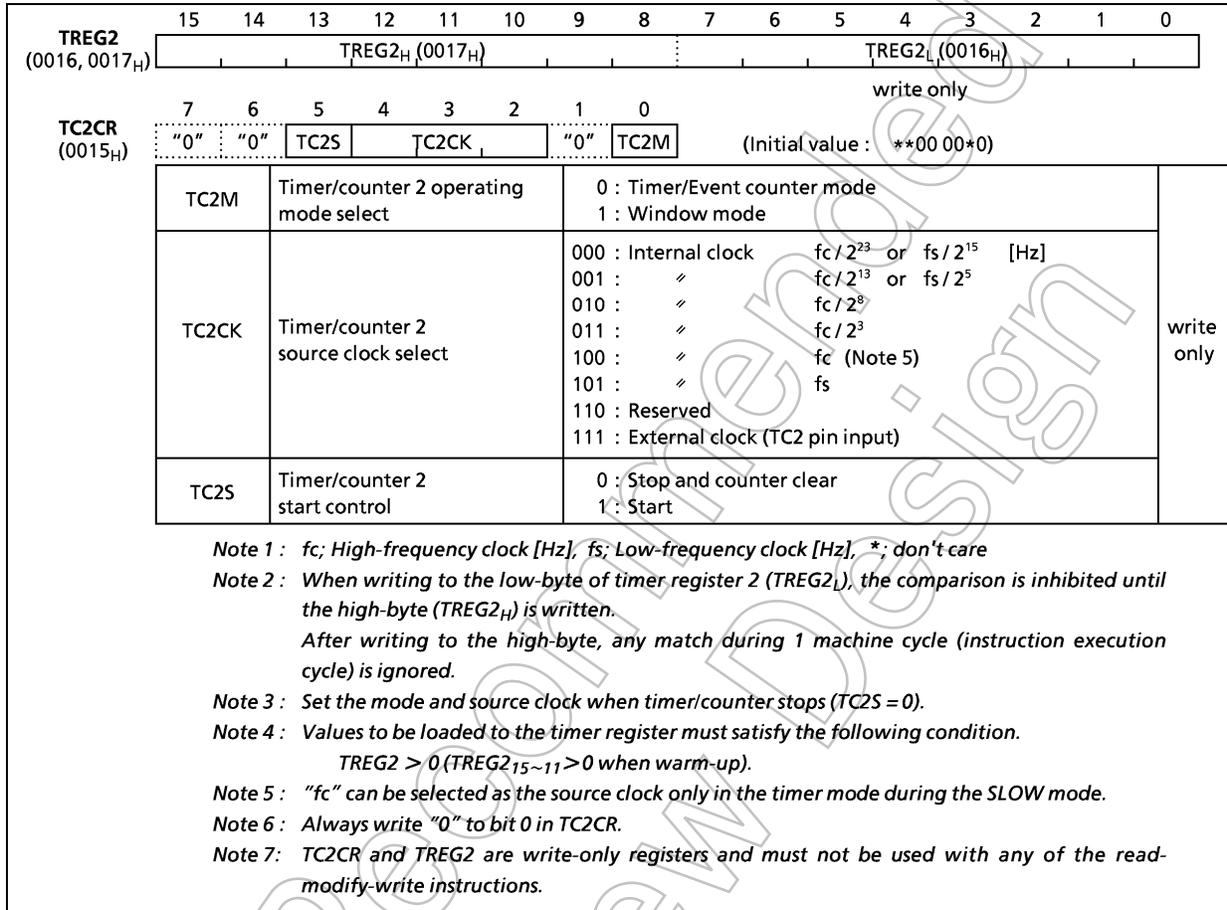
Figure 2-28. Timer Register 2 and TC2 Control Register
