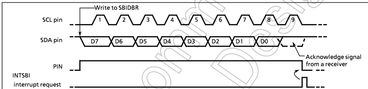
Figure 2-49. Example when BC = "000", ACK = "1" in Transmitter Mode
