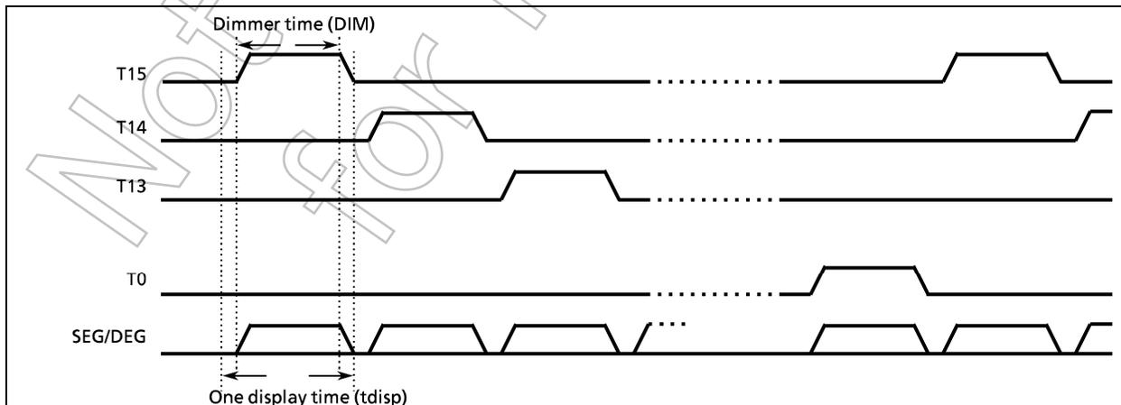
Figure 2-83. VFT Drive Waveform and Display timing
