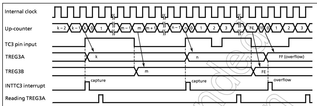
Figure 2-32. Timing Chart for Capture Mode (INT3ES = 0)
