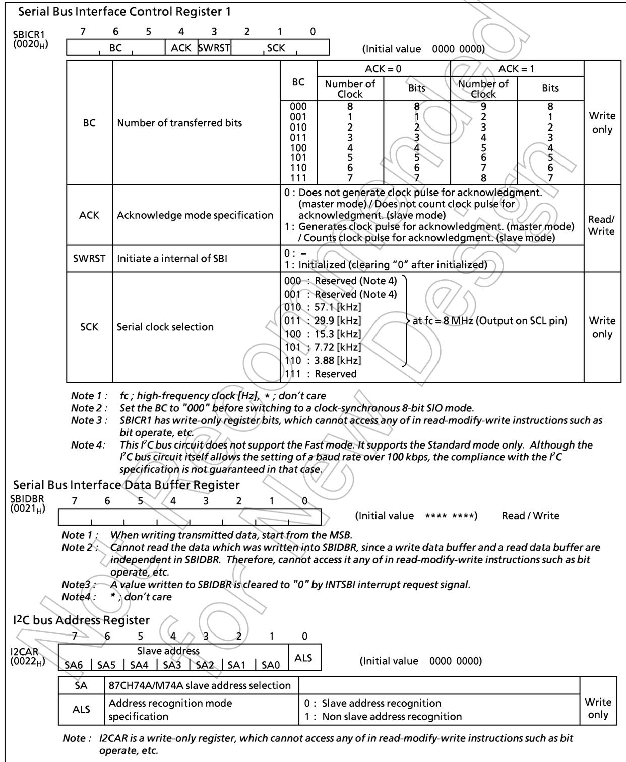
Figure 2-40. Serial Bus Interface Control Register 1 / Serial Bus Interface Data Buffer Register / I<sup>2</sup>C bus Address Register in the I<sup>2</sup>C bus Mode
