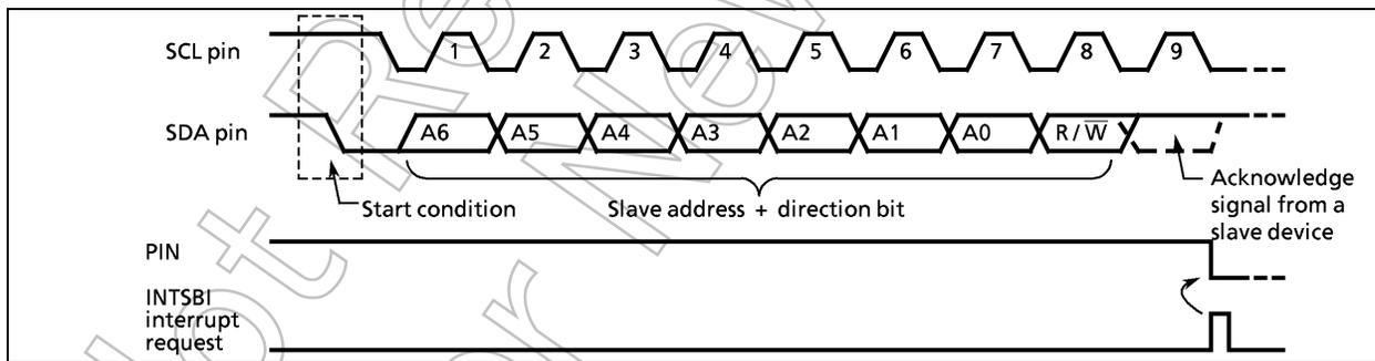
Figure 2-48. Start Condition Generation and Slave Address Transfer
