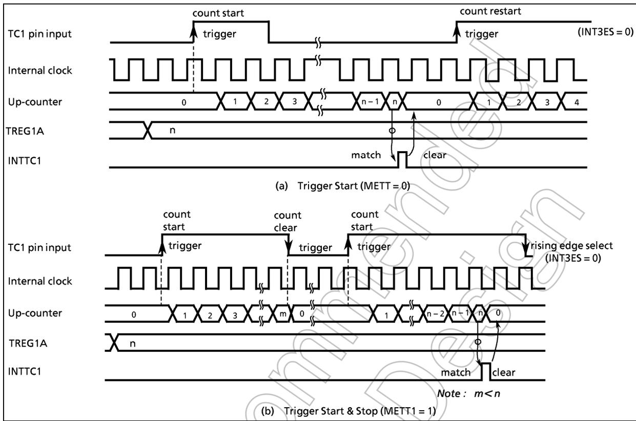
Figure 2-21. External Trigger Timer Mode Timing Chart
