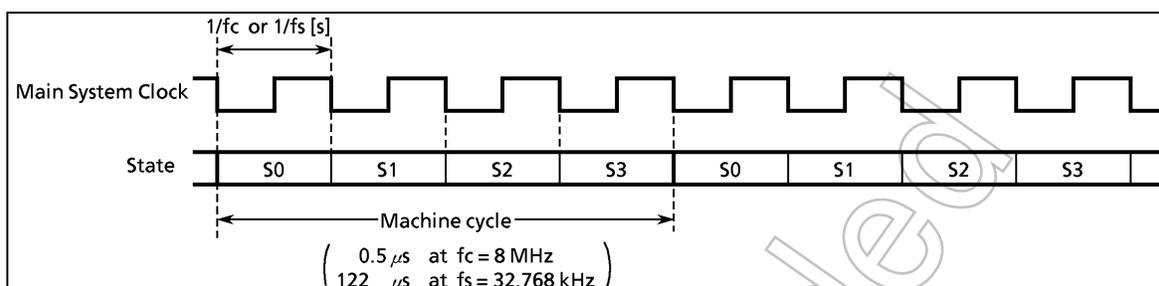
Figure 1-13. Machine Cycle
