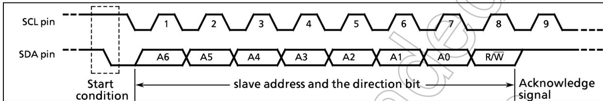
Figure 2-44. Start Condition Generation and Slave Address Generation
