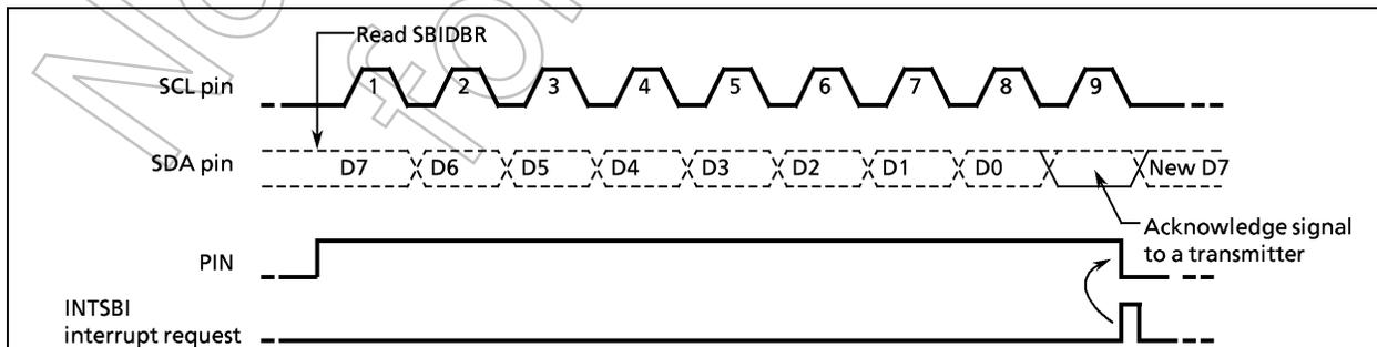
Figure 2-50. Example when BC = "000", ACK = "1" in Receiver Mode
