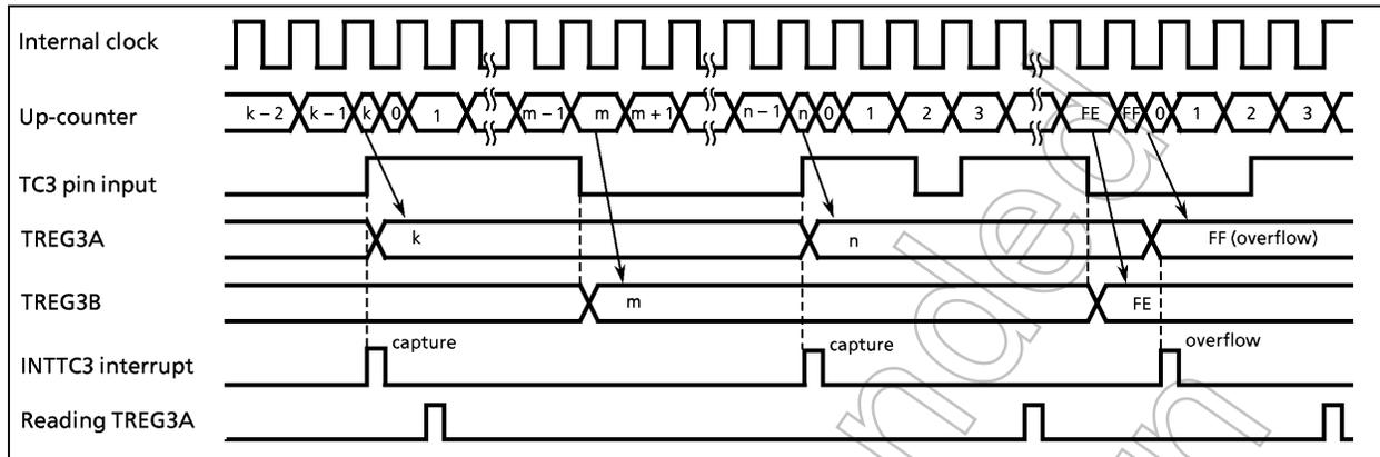
Figure 2-27. Timing Chart for Capture Mode (INT3ES = 0)
