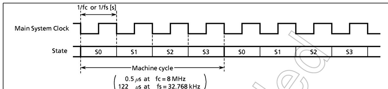
Figure 1-13. Machine Cycle
