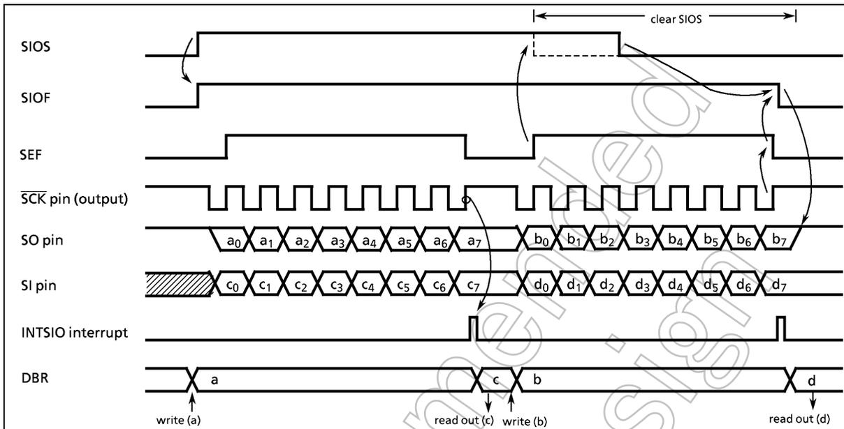
Figure 2-39. Transmit/Receive Mode (Example : 8-bit, 1word, internal clock)
