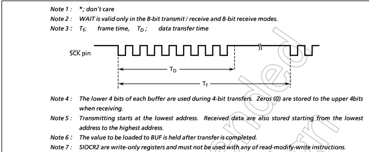
Figure 2-33. SIO Control Registers and Status Registers
