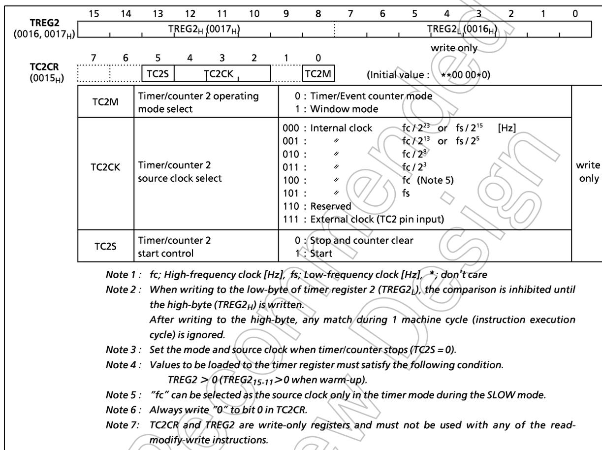
Figure 2-23. Timer Register 2 and TC2 Control Register
