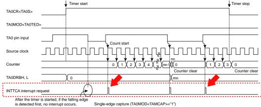
2. The timing diagram for double-edge capture indicates that no interrupt request occurs at the count start edge after the timer is started. This should be corrected so that an interrupt request occurs at the count start edge, as shown below.
