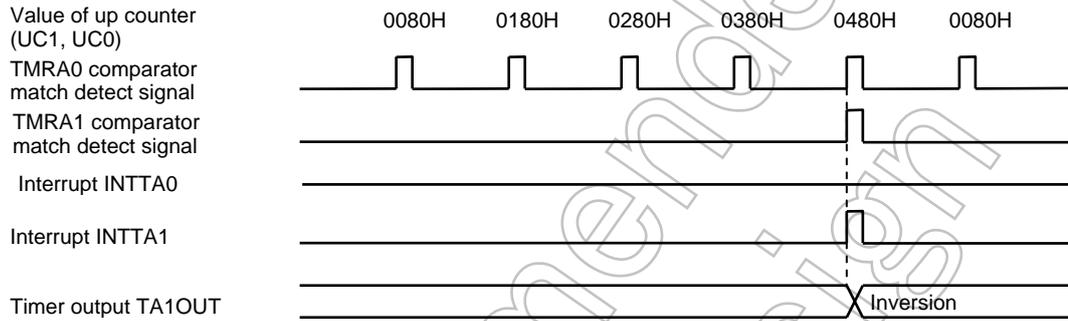
Figure 3.7.16 Timer Output by 16-Bit Timer Mode
