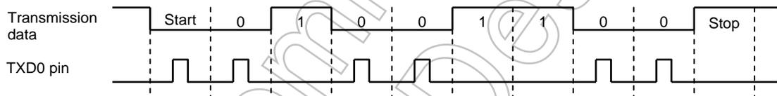
Figure 3.9.31 Transmission Example (SIO0)
