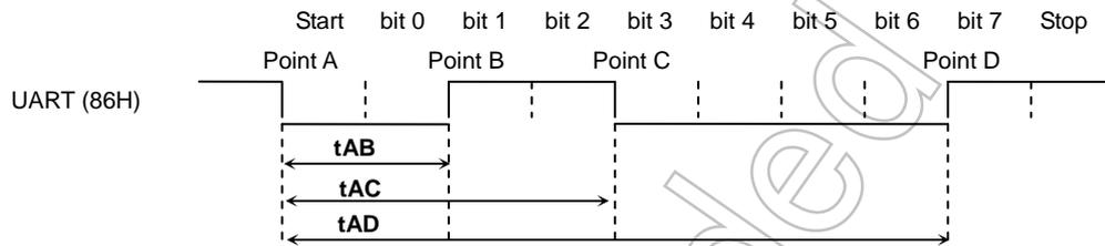
Figure 3.16.7 Data for Determining Serial Operation Mode
