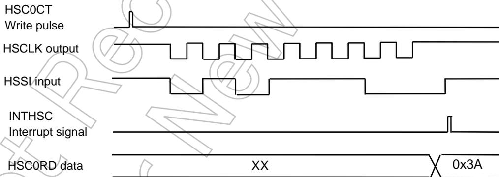
Figure 3.11.27 Example of UNIT receiving
