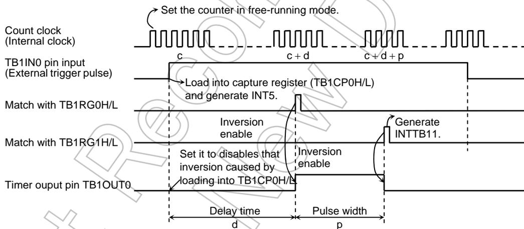
Figure 3.8.13 One-shot Pulse Output (with delay)
