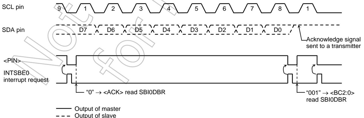
Figure3.10.21 Termination of Data Transfer in Master Receiver Mode
