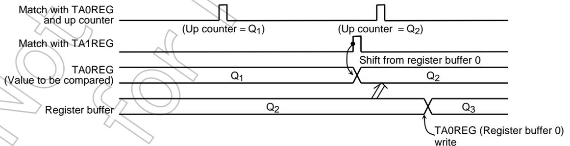
Figure 3.7.19 Operation of Register Buffer 0
