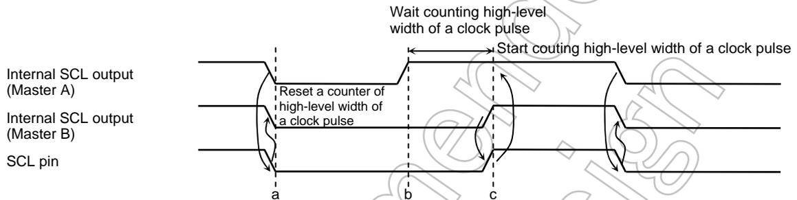
Figure 3.10.13 Clock Synchronization
