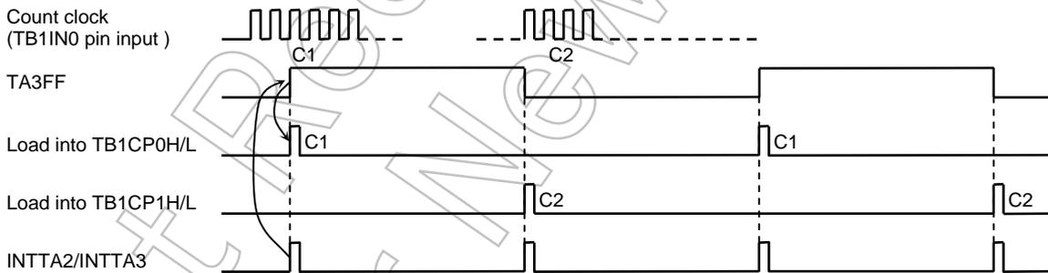
Figure 3.8.15 Frequency Measurement
