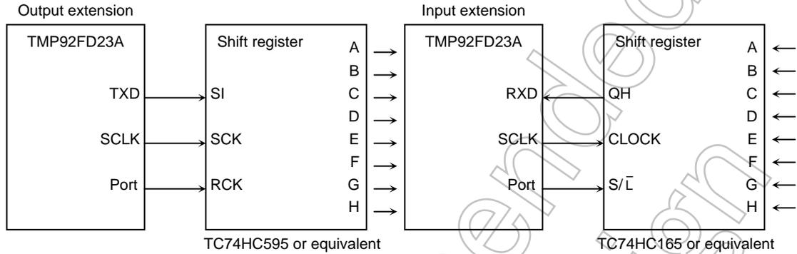
Figure 3.9.23 SCLK Output Mode Connection Example
