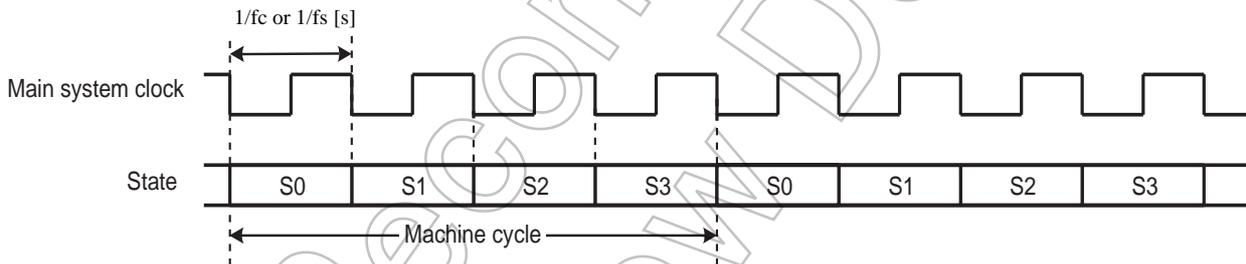
Figure 2-5 Machine Cycle
