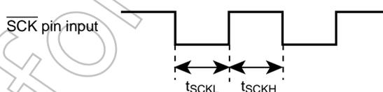
$t_{\text{SCKL}}, t_{\text{SCKH}} \geq 4/f_c$  (High-frequency clock mode)
