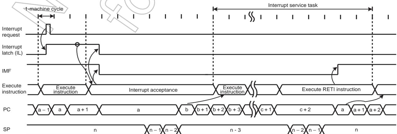
Note 1: a: Return address entry address, b: Entry address, c: Address which RETI instruction is stored
