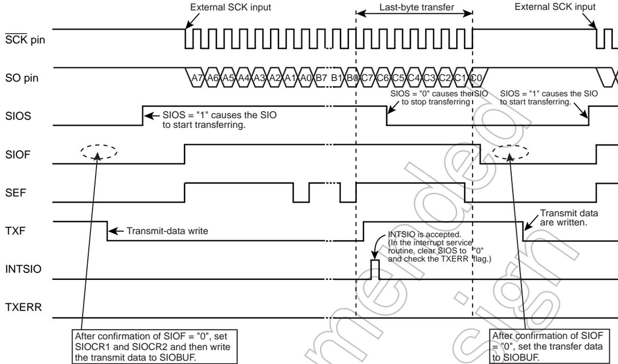
Figure 12-8 Transmit Mode Operation
