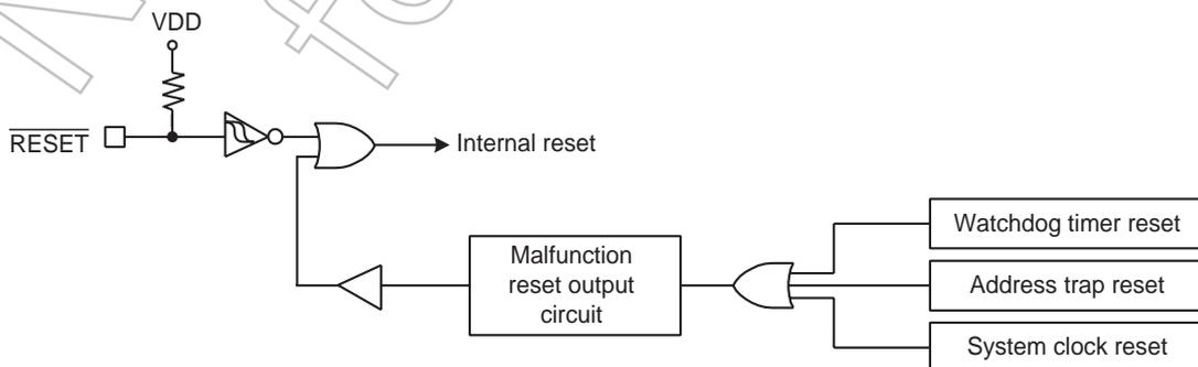
Figure 2-15 Reset Circuit
