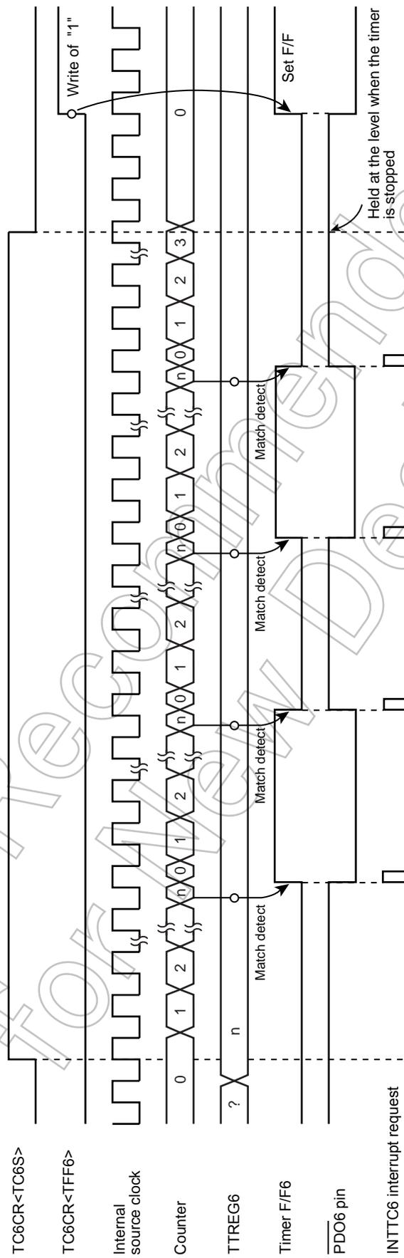
Figure 11-4 8-Bit PDO Mode Timing Chart (TC6)
