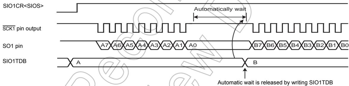
Figure 14-2 Automatic-wait Function (Example of transmit mode)
