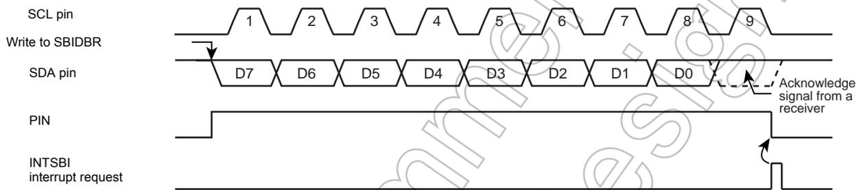
Figure 16-10 Example of when BC = "000", ACK = "1"
