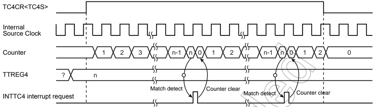
Figure 10-2 8-Bit Timer Mode Timing Chart (TC4)
