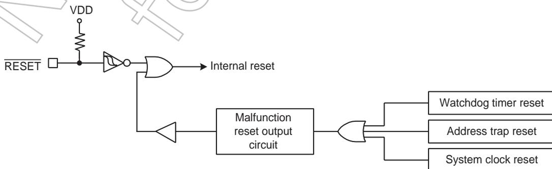
Figure 2-15 Reset Circuit
