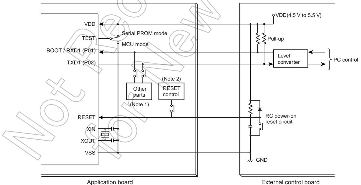
Figure 20-3 Example Connection for On-Board Writing
