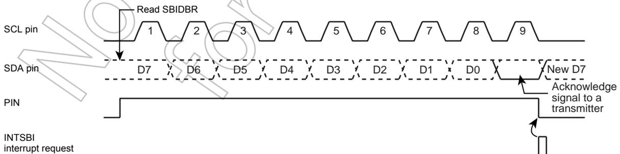
Figure 16-11 Example of when BC = "000", ACK = "1"
