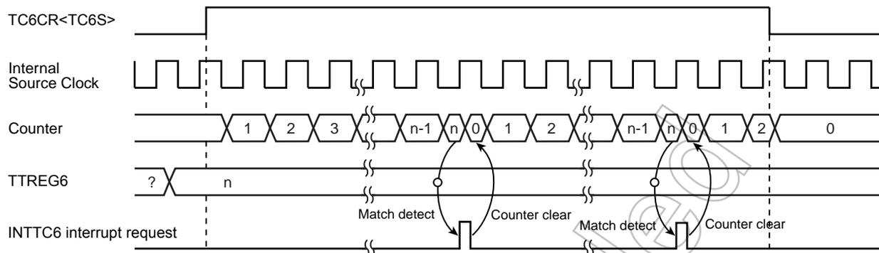
Figure 11-2 8-Bit Timer Mode Timing Chart (TC6)
