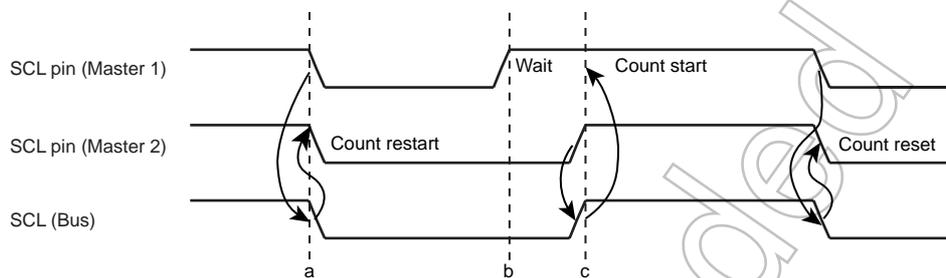
Figure 16-4 Clock Synchronization
