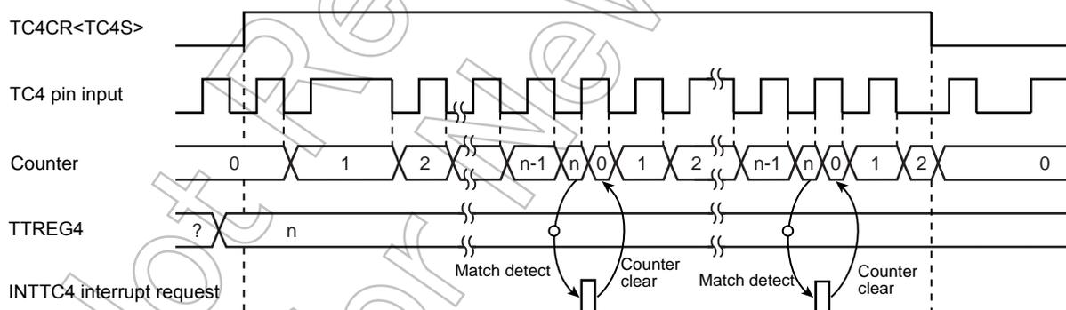
Figure 10-3 8-Bit Event Counter Mode Timing Chart (TC4)
