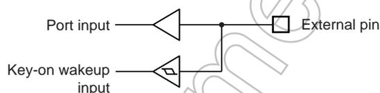
Figure 18-2 Key-on Wakeup Input and Port Input
