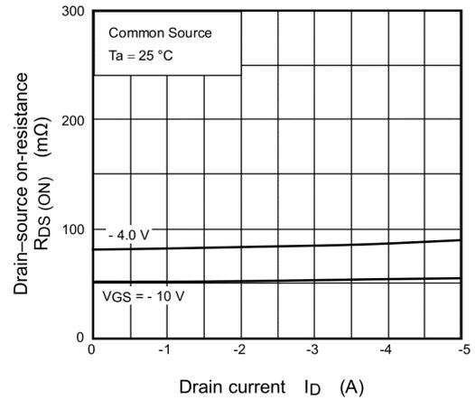
Fig. 7.4  $R_{DS(ON)} - I_D$
