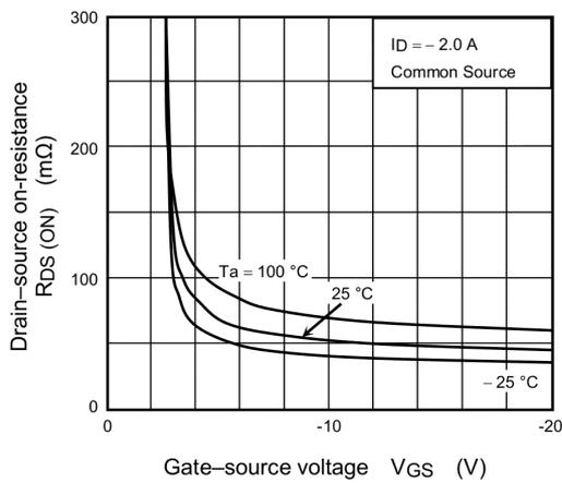
Fig. 7.3  $R_{DS(ON)} - V_{GS}$
