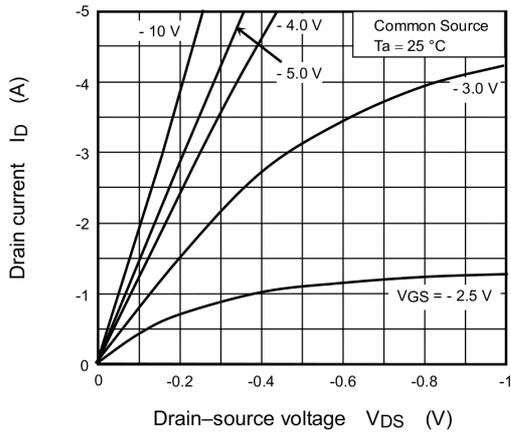
Fig. 7.1  $I_D - V_{DS}$
