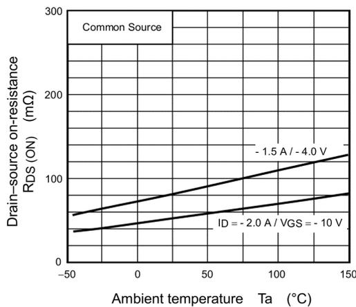
Fig. 7.5  $R_{DS(ON)} - T_a$
