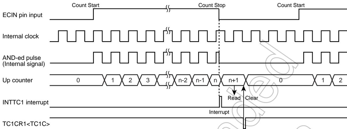
Figure 8-4 Pulse width measurement mode timing chart
