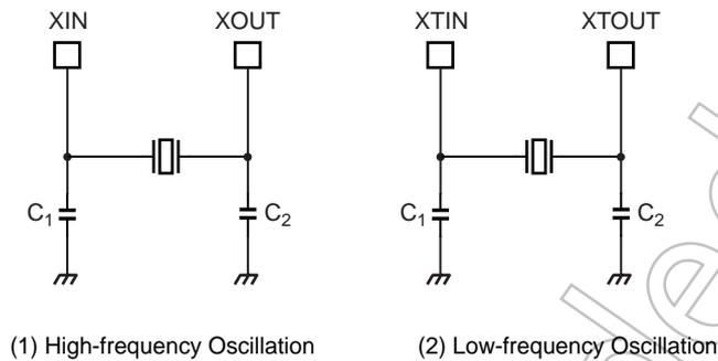
Note 1: A quartz resonator can be used for high-frequency oscillation only when  $V_{DD}$  is 2.7 V or above. If  $V_{DD}$  is below 2.7 V, use a ceramic resonator.
