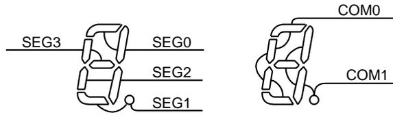
Figure 13-7 Example of COM, SEG Pin Connection
