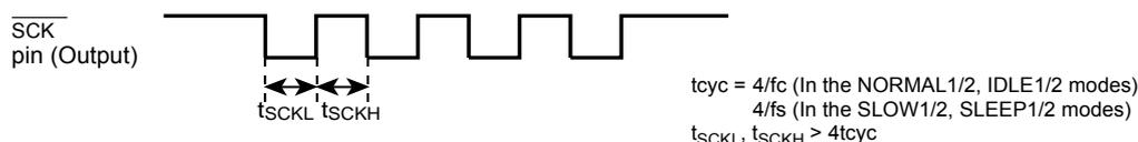
Figure 10-4 External clock pulse width
