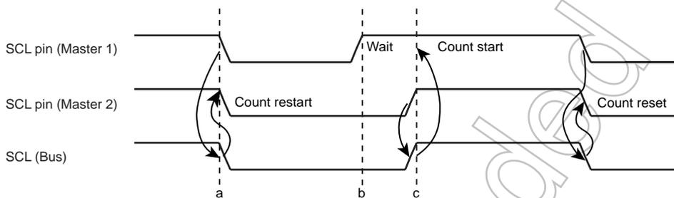
Figure 16-4 Clock Synchronization
