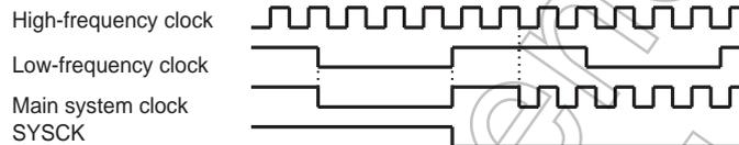
Example :Switching from the SLOW1 mode to the NORMAL2 mode (fc = 16 MHz, warm-up time is 4.0 ms).
