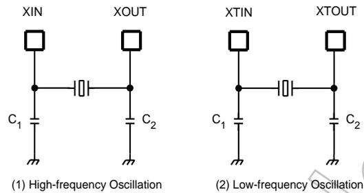
Note 1: A quartz resonator can be used for high-frequency oscillation only when VDD is 2.7 V or above. If VDD is below 2.7 V, use a ceramic resonator.
