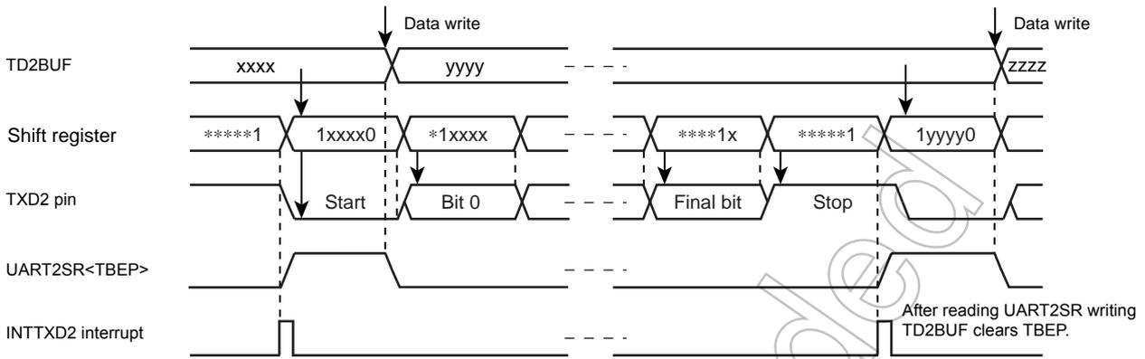
Figure 13-9 Generation of Transmit Data Buffer Empty
