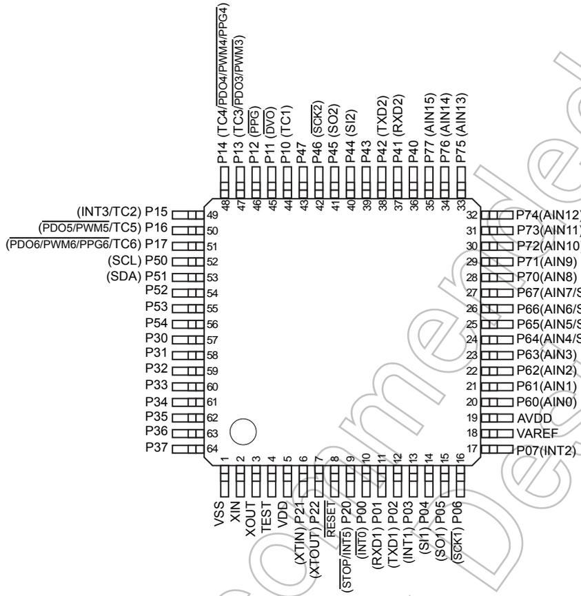
Figure 1-1 Pin Assignment
