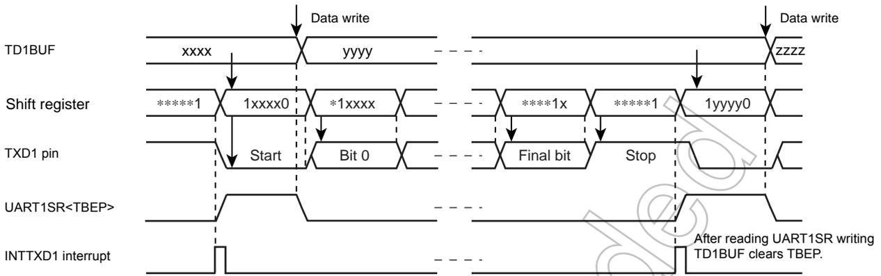
Figure 12-9 Generation of Transmit Data Buffer Empty
