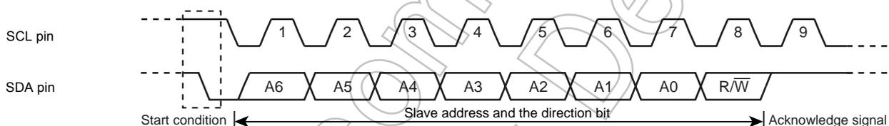
Figure 16-5 Start Condition Generation and Slave Address Generation
