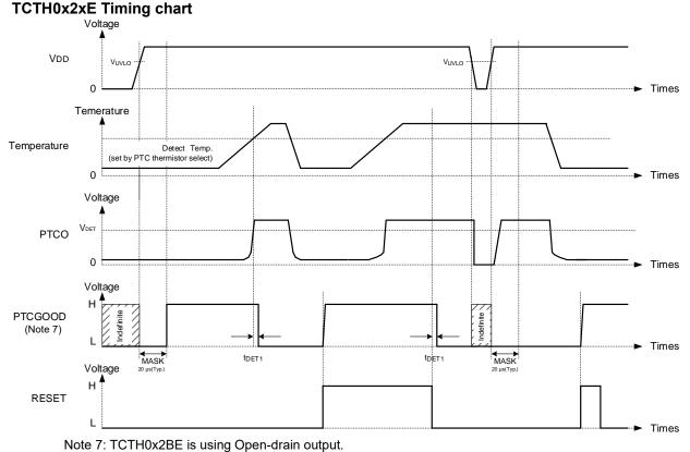
Therefore, PTCGOOD pin of TCTH0x2BE outputs High-impedance instead of "High".
