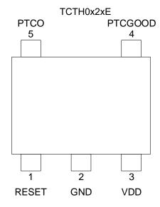
Note4: All GND pin must connect to the system GND.
