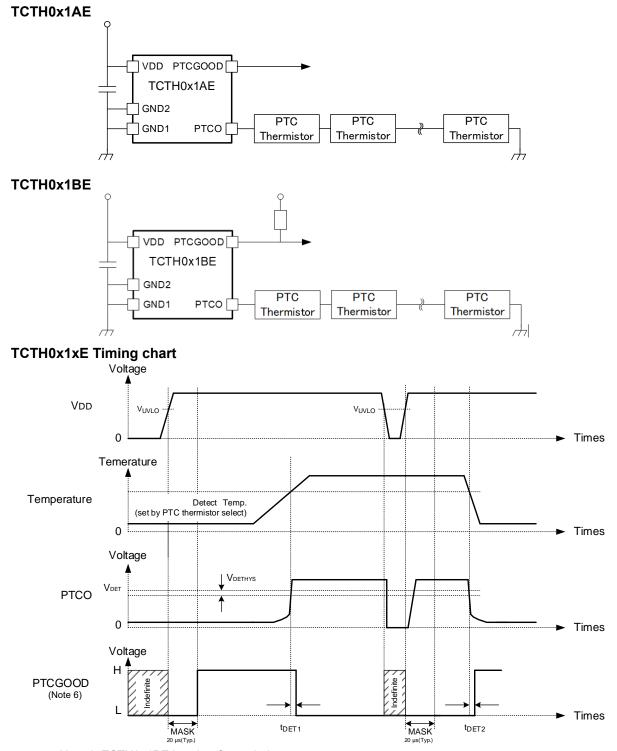
Note 6: TCTH0x1BE is using Open-drain output. Therefore, PTCGOOD pin of TCTH0x1BE outputs High-impedance instead of "High".
