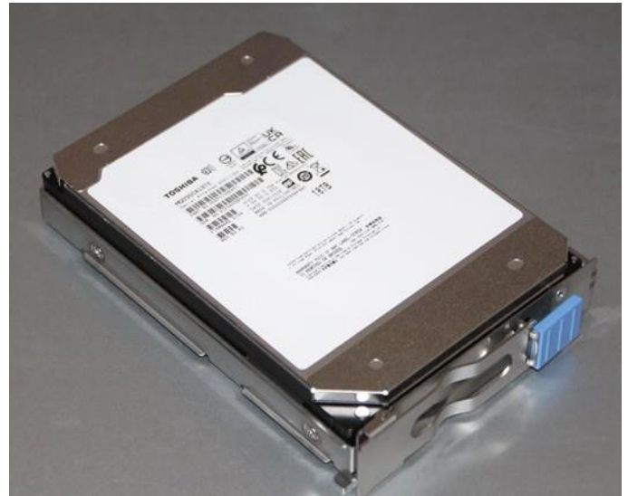
Picture 3: Toshiba HDD MG09SCA18TE in PROMISE tray.
