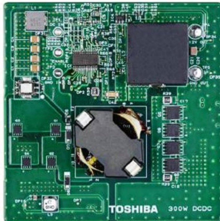
Figure 1. Physical evaluation circuit used to investigate secondary-side losses on a 300 W DC-DC converter.
