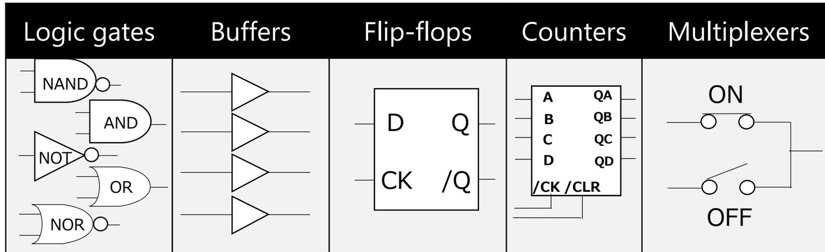
Analog switches that connect or disconnect the conducting path of an analog signal are also classified as logic ICs.
