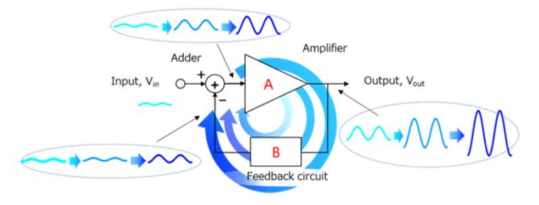
Let the open-loop gain of the op-amp be  $A_V$  and the feedback factor be B. Then, the transfer function of a feedback circuit is expressed as follows. Both  $A_V$  and B are complex numbers.
