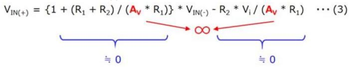
Because the output impedance is zero, we obtain  $V_{IN(+)} = V_{IN(-)}$  from Equation 3. Hence, the voltage at the  $V_{IN(-)}$  input is equal to that of the  $V_{IN(+)}$  input connected to GND. In this case, the condition of the  $V_{IN(-)}$  input is called a virtual short.
