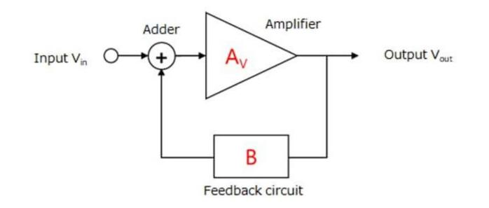
The amplifier amplifies the input signal and outputs an amplified signal. Part of the output is returned to the input of the amplifier via the feedback circuit and the adder.
