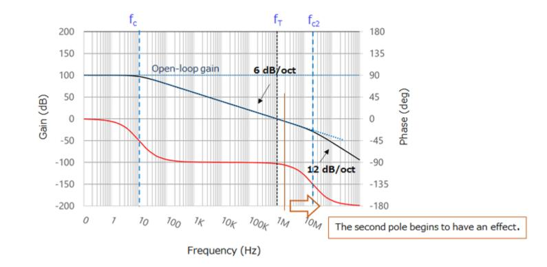
In order to avoid abnormal oscillation, an op-amp should be used in the frequency range ( $f_c$  to  $f_{c2}$ ) in which the open-loop gain decreases at a rate of 6 dB per octave. Note, however, that, at a frequency close to  $f_{c2}$ , an op-amp is affected by a second pole, causing a power loss and a phase delay. To avoid its effects completely, the closed-loop bandwidth ( $f_{CL}$ ) should be less than one-fifth of  $f_{c2}$ .
