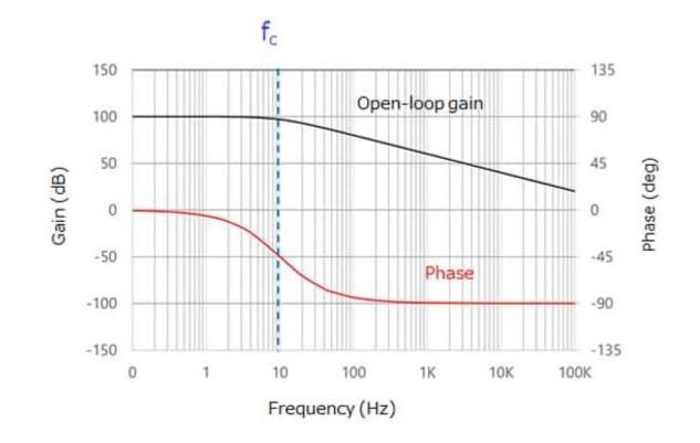
In reality, an op-amp has multiple poles. The cut-off frequency ( $f_c$ ) shown in Figure is called the main pole. The frequency pole at  $f_{c2}$  close to the unity gain cross frequency ( $f_T$ ) is called a second pole. Although there are more poles at higher frequencies, they do not cause any practical problem.
