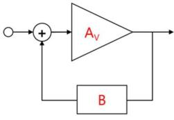
The input ( $V_{in}$ ) and the output ( $V_{out}$ ) have the following relationship. This relationship is called a closed-loop gain (represented as  $G_{CL}$  in dB scale and  $A_{CL}$  in linear scale). The 20 log rule is used to convert a linear voltage gain into a decibel voltage gain: G = 20 × log A.
