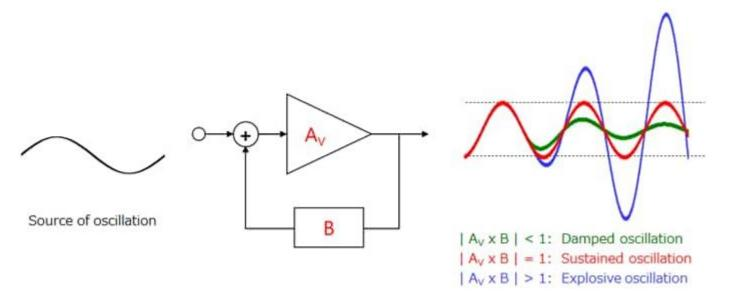
A sustained oscillation occurs when the loop gain ( $A_V \times B$ ) satisfies the following condition (i.e., the denominator of the transfer function becomes zero). This condition is called the Barkhausen condition for oscillation (or simply oscillation condition).
