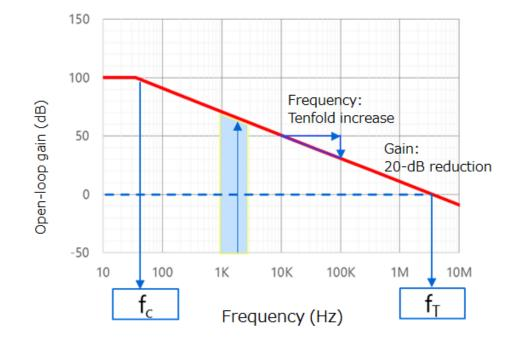
Now, let's consider what occurs when an input signal with a frequency of  $2\pm1$  kHz is applied to an op-amp that has frequency characteristics as shown in Figure. In the case of an op-amp under this condition, the gain at 3 kHz is roughly 10 dB lower than the gain at 1 kHz. Normally, the op-amp cannot be used under this condition. Negative feedback solves this issue.
