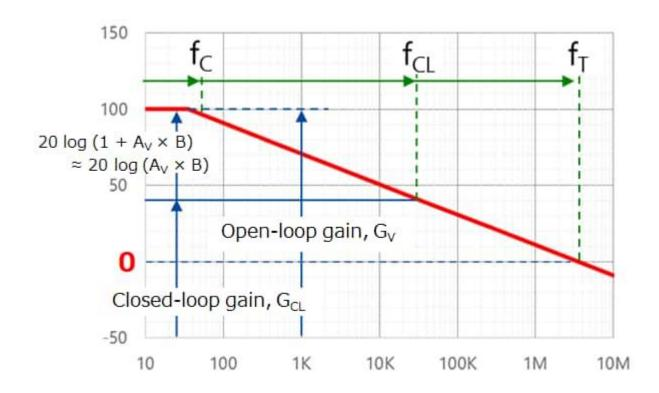
An op-amp is normally used with a feedback circuit as shown in Figure. There are two types of feedback, positive and negative, as described in Section 1. When an op-amp is used as an amplifier, it is configured for negative feedback. Care is required as to the oscillation of a feedback circuit.
