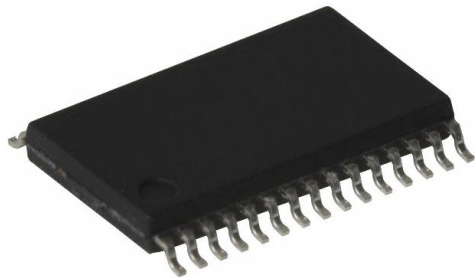
SSOP30 package ( 10.2 x 7.6 x 1.6 mm )
