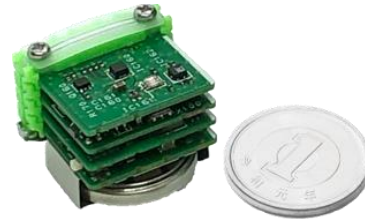
Fig. 3. Photograph of proposed module consisting of four leaf PCBs.
