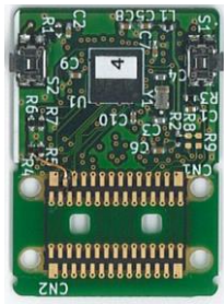
Fig. 8. 32-bit MCU leaf PCB with 58-pin bus connection.
