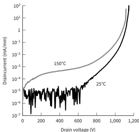
**Figure 7. Breakdown characteristics of GaN MOSFET**
