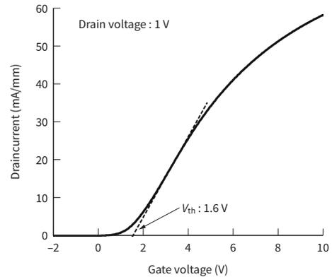
**Figure 5. Transfer characteristics of GaN MOSFET**
