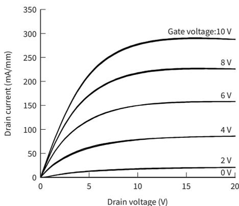
**Figure 4. Output characteristics of GaN MOSFET**
