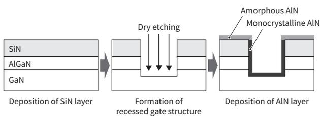
match the crystallinity between the AlN and GaN layers. The other AlN layers on the SiN layer are deposited as amorphous layers. We have developed a process technology to selectively control the crystallinity of the AlN layers as described above.
