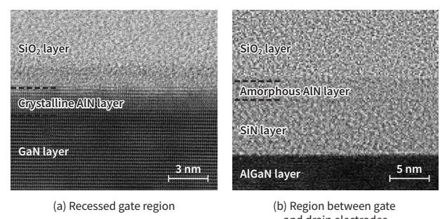
**Figure 3. Cross-sectional TEM images of AlN film fabricated areas**
