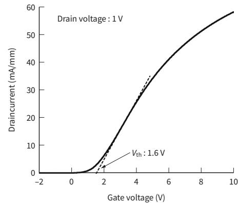
**Figure 5. Transfer characteristics of GaN MOSFET**
