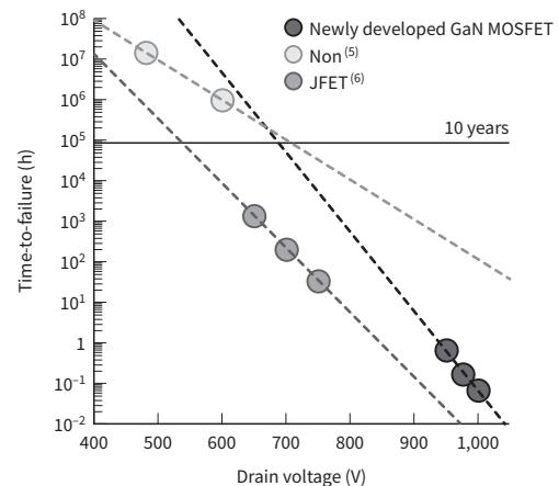
**Figure 8. Results of reliability tests when high voltage was applied at high temperature**
