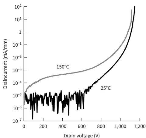
**Figure 7. Breakdown characteristics of GaN MOSFET**
