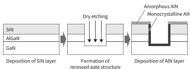
**Figure 2. Flow of processes for fabrication of recessed gate structure**
