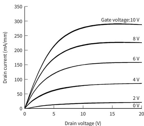
**Figure 4. Output characteristics of GaN MOSFET**
