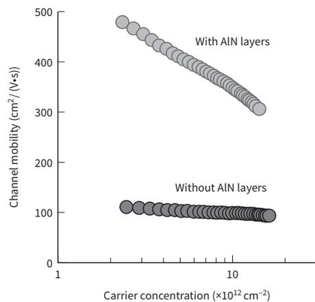
**Figure 6. Dependence of channel mobility on carrier density**
