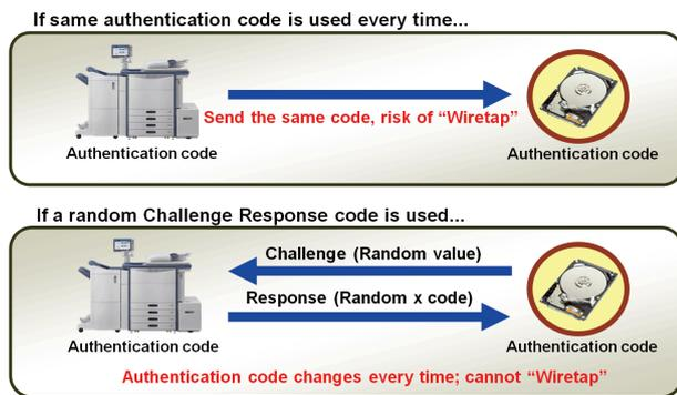
The Wipe2 SED is able to judge the authentication code from a Wipe2 enabled host by comparing the completing the pre-determined challenge and response protocol process inside the secure SED device.
